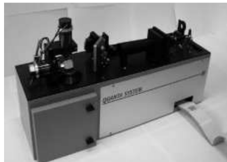
Fig. 12. The laser induced fluorescence detection system built by Quanta System; on the left side one can notice the two galvanometric motors that are driving the deflection mirrors of the laser beam [31].
