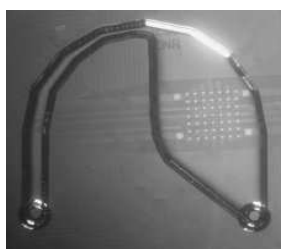
Fig. 8. The 200 \mu\text{m} deep reservoir etched in glass, covering the electrodes array.
