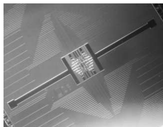
Fig. 6. The polyimide reservoirs; Stereo micrograph x 10 [30].
