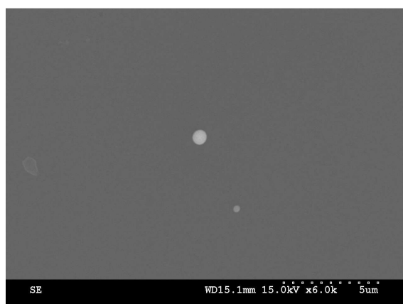
Fig. 2. A surface SEM image of a PLD Ti thin film grown on Si.
