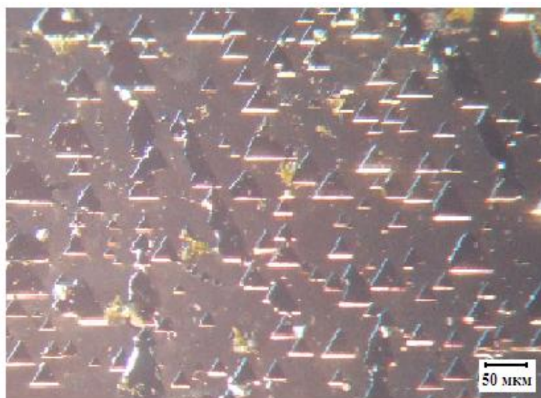
Fig. 4. Formation of embryos on the Si (111) substrate in the initial stage of epitaxy of the solid solution (\text{Si}_2)_{1-x}(\text{GaP})_x (colour online)
