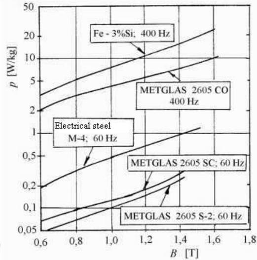
Fig. 14. Total losses for several soft magnetic materials versus magnetic flux density [31].
