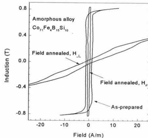
Fig. 15. DC hysteresis loops for an amorphous strip 71%Co-4%Fe-15%B-10%Si, before and after annealing in longitudinal and transversal fields close to saturation value.
