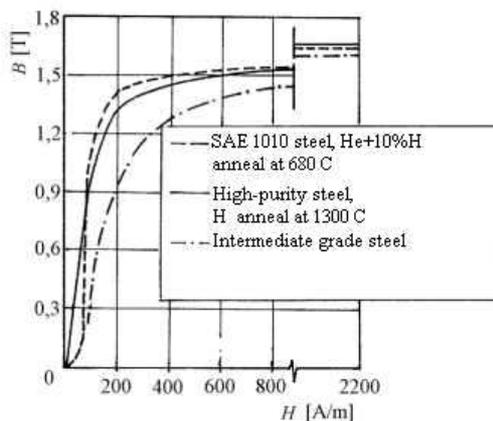
Fig. 8. Initial magnetization curves for two iron steels of high purity annealed in hydrogen atmosphere, and for usual steels [30].
