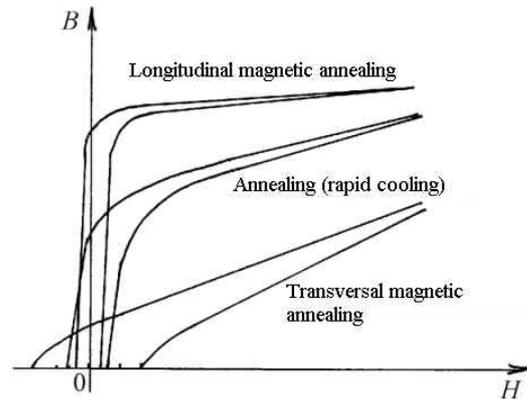
Fig. 2. Typical hysteresis loops for amorphous alloys subjected to annealing.
