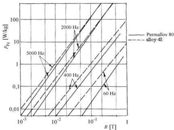
Fig. 10. Total iron losses versus magnetic flux density and its frequency for two types of sheets made from Ni-Fe alloys,  $D = 0.35\text{mm}$ .
