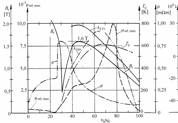
Fig. 9. Fe-Ni alloys properties versus their nickel content.
