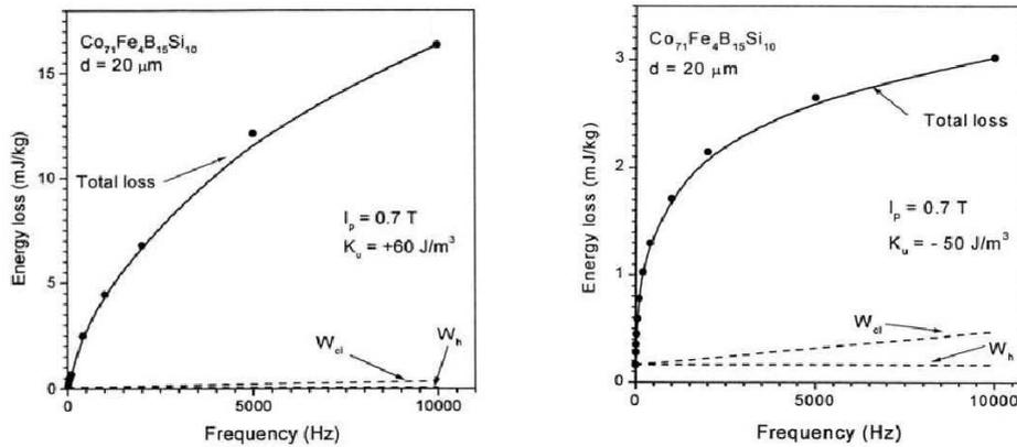
Fig. 16. Energy losses per cycle versus frequency, for amorphous Co based amorphous strips, annealed in longitudinal (a) and transversal field (b), close to saturation: (a)  $K_u = 60 \text{ J/m}^3$ ; (b)  $K_u = -50 \text{ J/m}^3$ . The points correspond to the experimental measurements [15], the continuous lines represent the total losses and the dotted lines the classical and the hysteresis losses, respectively.
