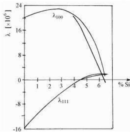
Fig. 4. The values of magnetostrictive constants  $\lambda_{001}$  and  $\lambda_{111}$  of the Fe-Si alloys versus Si content; the lower curves in the interval 4 - 7 wt. % Si correspond to a slow cooling.
