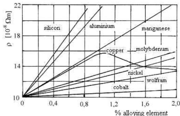
Fig. 3. Variation of the electrical resistivity of Fe-based alloys vs. addition element.
