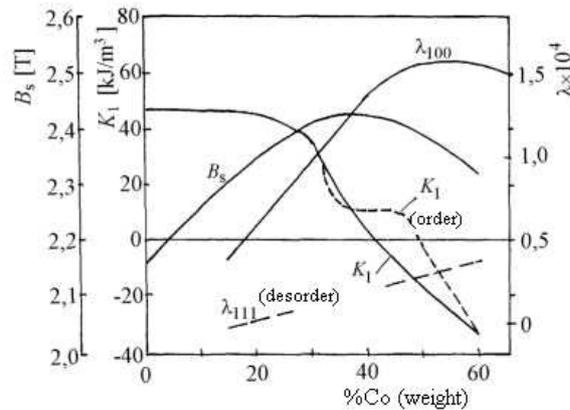
Fig. 11. Magnetic characteristics of Fe-Co alloys versus cobalt content, at room temperature [2].
