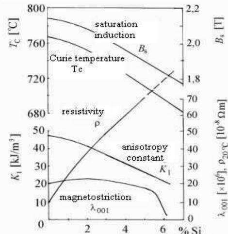
Fig. 5. The variation of the electric and magnetic properties of Fe - Si alloys in respect with their Si content (©1971 IEEE).
