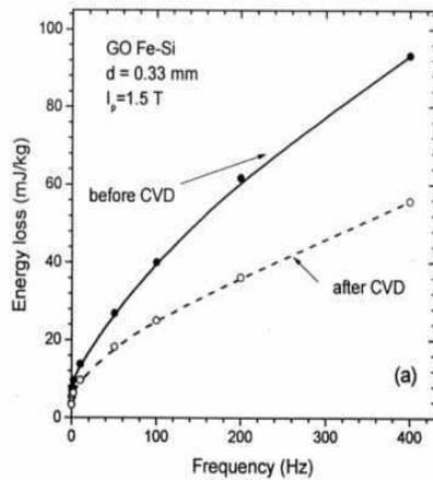
Fig. 6. Energy losses per cycle versus the excitation frequency for the G.O. sheets before and after the treatment by CVD with  $\text{SiCl}_4$ , that leads to the Si content increase from 3% to 6,5% [15].
