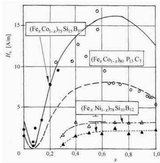
Fig. 13. Dependence of the coercive field on the composition, for several magnetic amorphous alloys.
