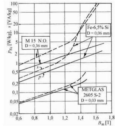
Fig. 7. Losses and excitation power at 60Hz, versus the magnetic flux, for some soft magnetic materials: Fe-Si M-15 N.O. steel, Fe-6,5%Si steel obtained by rapid cooling and amorphous METGLAS 2605S-2. Under 1,6T, the M-4 G.O. alloys and Fe-6,5%Si have almost identical losses.
