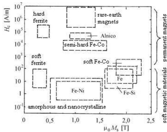
Fig. 1. Main classes of soft magnetic materials [2].
