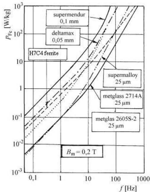
Fig. 12. Iron losses, at high frequencies, of some materials [3]. The metallic samples of reduced thicknesses can still be used.
