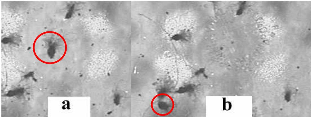
Fig. 4. Spores of *Chaetomium* sp. (a) have been slowly displaced by laser cleaning (b).
