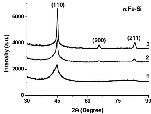
Fig. 3. X-ray diffraction patterns after different annealings: 1) 510°C /0.5h, 2) 530 °C/1h, 3) 540 °C/1h.
