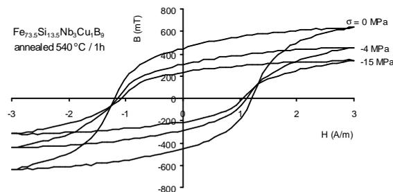
Fig. 4. The influence of compressive stress  $\sigma$  on the hysteresis loop of Finemet type  $\text{Fe}_{73.5}\text{Si}_{13.5}\text{Nb}_3\text{Cu}_1\text{B}_9$  alloy in nanocrystalline state (annealed in 540 °C for 1 h).
