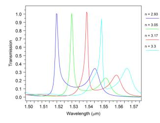
Fig. 7. Output spectra of the proposed filter for different refractive indices.
