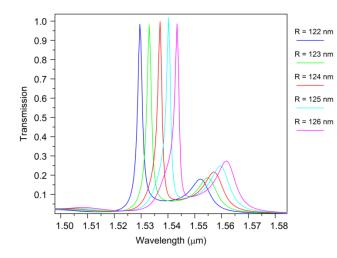
Fig. 5. Output spectra of the proposed filter for different Radius (R)
