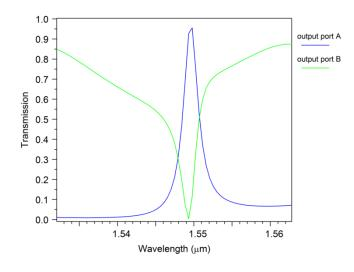
Fig. 3. Output spectrum of the filter.
