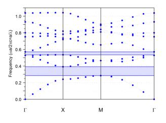
Fig 1. Band structure of fundamental photonic crystal.
