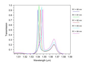
Fig. 6. Output spectra of the suggested filter for different defect Radius (R1).
