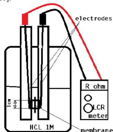
Fig. 3 Proton conductivity measurement installation scheme
