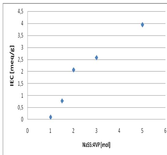
Fig. 5. Ion exchange capacity function of copolymer NaSSA-4VP initial monomers mole ratio
