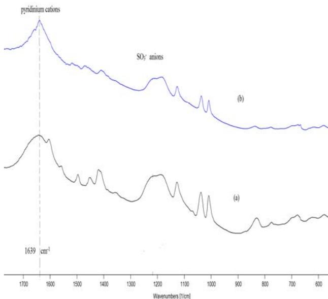
Fig. 4 MIR spectra (a) Copolymer NaSSA-4VP2, (b) Membrane SSA-4VP2
