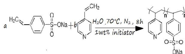
Fig. 1 Synthesis of poly(styrene sulfonic acid-co-4-vinylpyridine) copolymer through free radical polymerization ; a-mol of 4-NaSSa, b-mol of 4-VP
