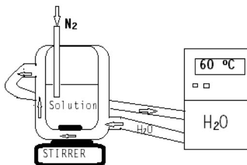
Fig. 2. Installation scheme of free radical polymerization.
