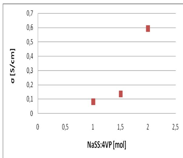
Fig. 7 Proton conductivity function of copolymer NaSSA-4VP initial monomers mole ratio
