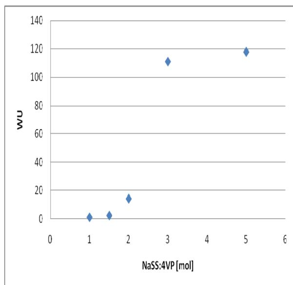
Fig. 6 Water function of copolymer NaSSA-4VP initial monomers mole ratio
