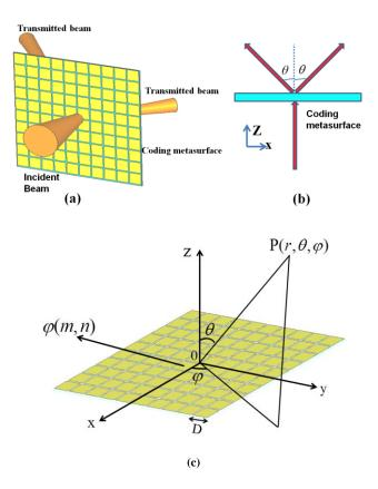
Fig. 1. (a) Schematic of proposed beam splitter by transmission-type coding metasurface (b) Top view of beam splitter by transmission-type coding metasurface (c) Schematic of coding metasurface, which contains N×N equal-size lattice with dimension D; each lattice is occupied by "1" or "0" digital elements
