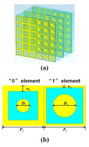
Fig. 2. (a) Schematic of the transmission-type coding metasurface that consist of three metallic layers and three polyimide spacers (b) Configuration of "0" and "1" elements and their dimensions are  $P_1=P_2=140 \ \mu m$ ,  $w_1=8 \ \mu m$ ,  $w_2=20 \ \mu m$ ,  $D_1=80 \ \mu m$ ,  $D_2=46 \ \mu m$ , respectively
