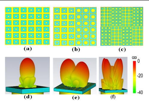
Fig. 5. (a-c) Transmission-type coding metasurface with different sequences: (a) 000000.../000000..., (b) 000111.../000111...
