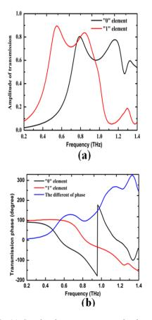
Fig. 3. (a) Simulated transmission amplitude of "0" and "1" digital elements (b) Simulated transmission-phase and their difference phase of "0" and "1" digital elements
