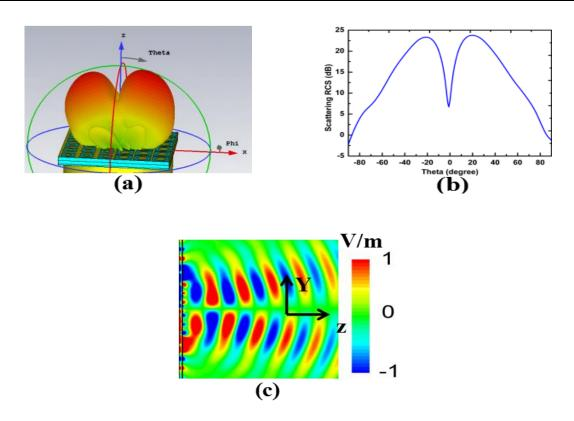
Fig. 4. (a) Simulated 3D field patterns of the coding metasurface under the normal incidence at 0.95 THz (b) Simulated 2D far-field patterns in the XOZ plane of the coding metasurface (c) Near electric field distribution of the effect on the YOZ plane at 0.95 THz
