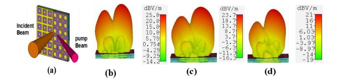
Fig. 6. (a) Schematic of optically controlled terahertz coding metasurface (b-d) The transmission two beams of 000111.../000111...coding metasurface for silicon with different conductivity at 0.95THz (b)  $\sigma = 1s/m$  (c)  $\sigma = 1 \times 10^4 s/m$  (d)  $\sigma = 3 \times 10^4 s/m$
