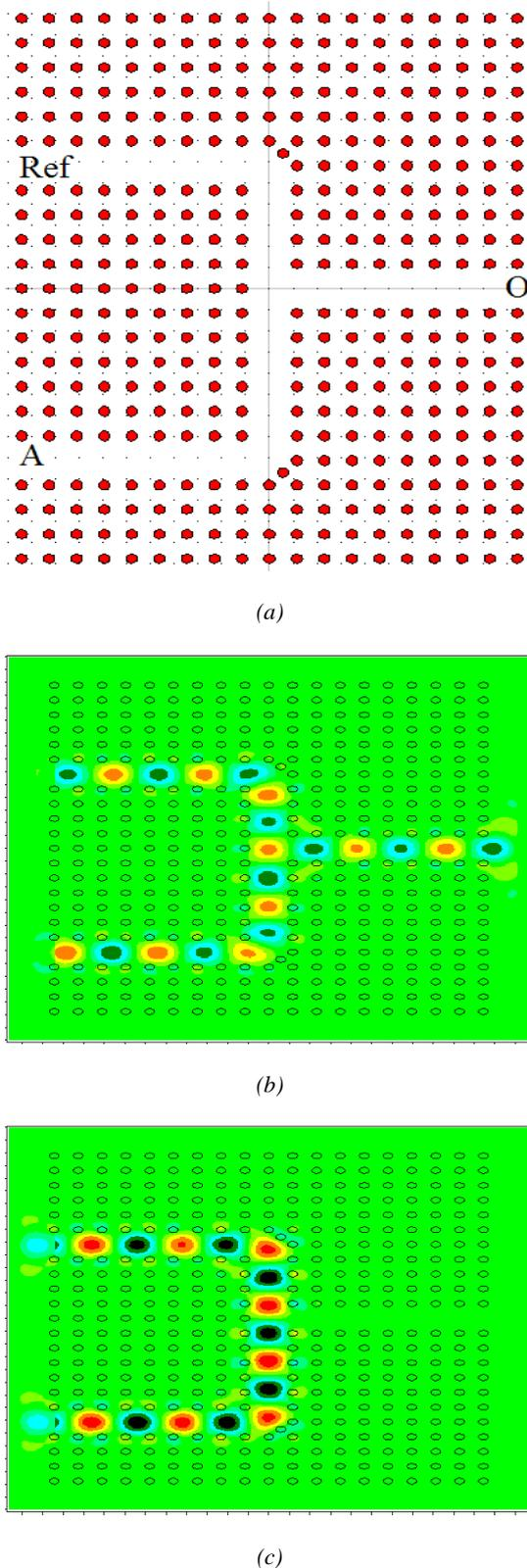
Fig. 3. (a) The optical NOT and its optical behavior when A is at logic (b) 0 and (c) 1 (color online)
