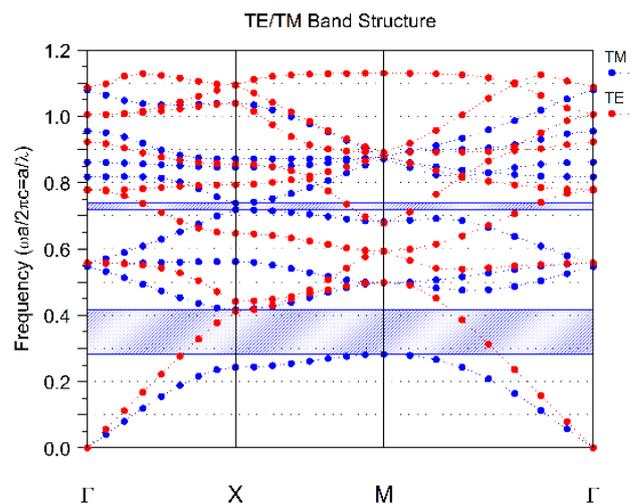
Fig. 1. The band structure diagram of the PhC (color online)
