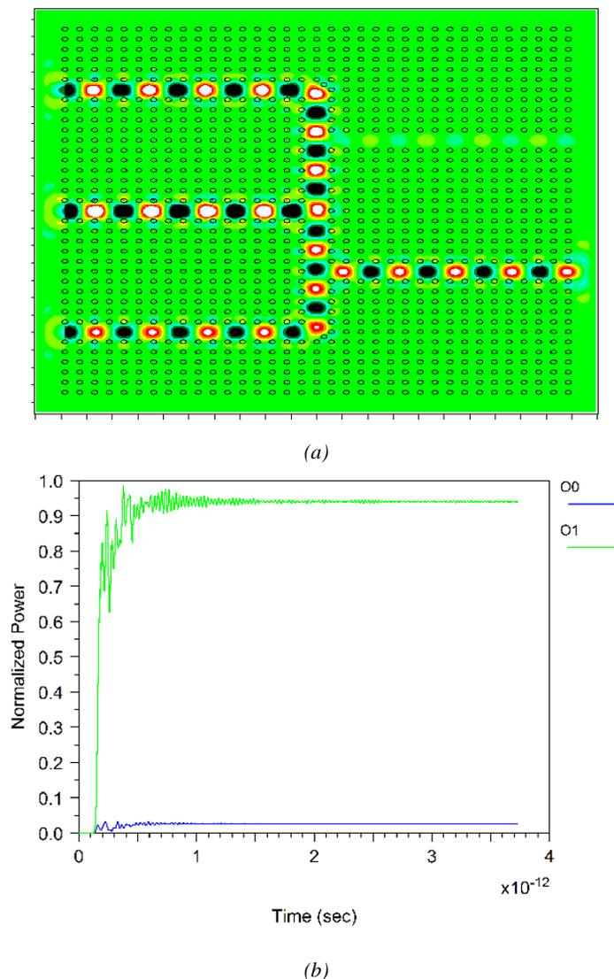
Fig. 6. (a) The optical behavior and (b) the time response diagram of the decoder when A is at logic 1 (color online)
