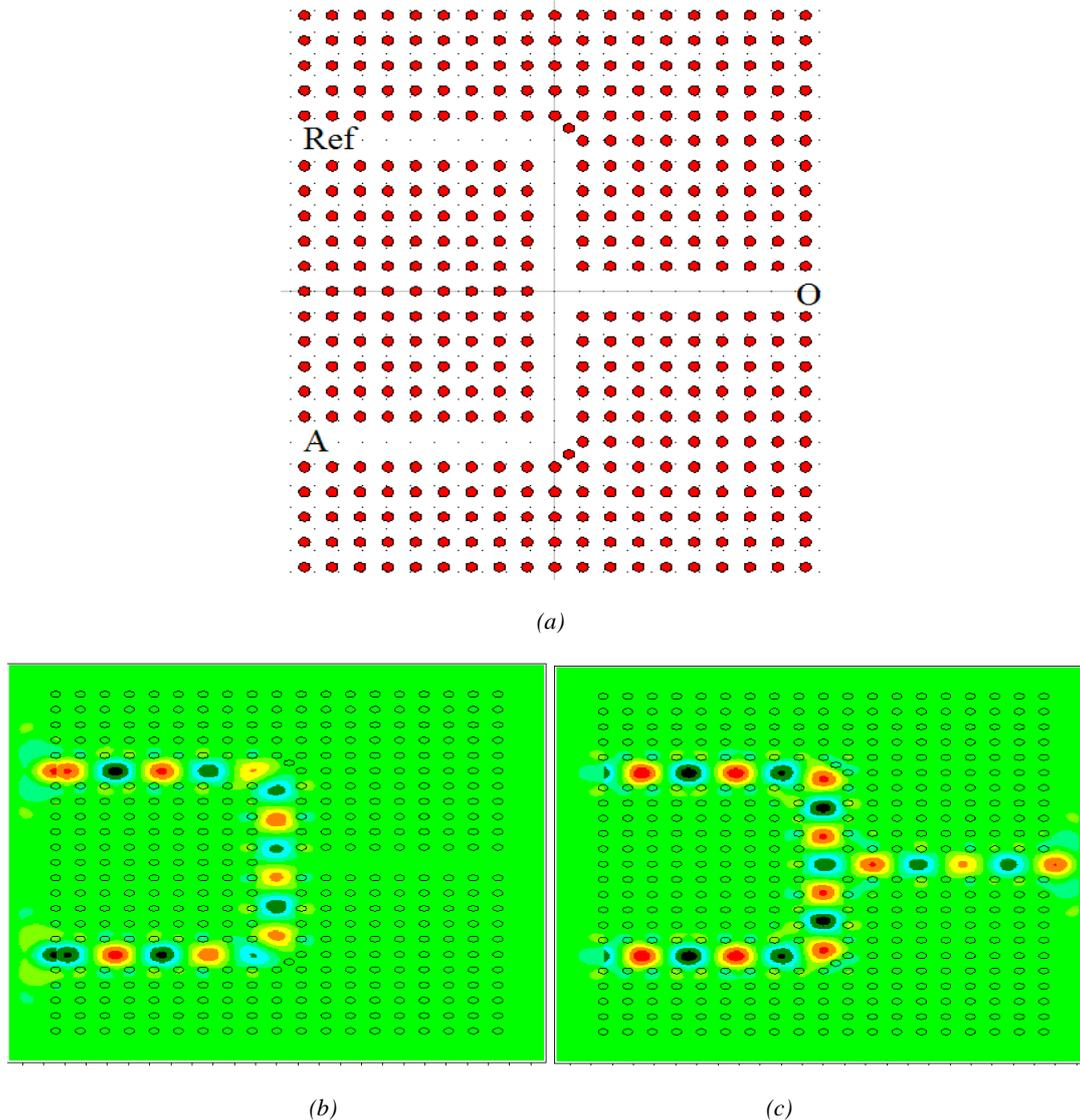
Fig. 2. (a) The optical buffer and its optical behavior when A is at logic (b) 0 and (c) 1 (color online)
