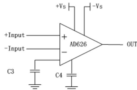
Fig. 5. Signal amplifying circuit diagram
