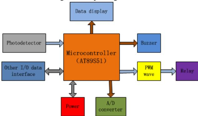
Fig. 7. The block diagram of micro controller
