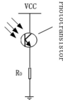
Fig. 4. The photoelectric conversion circuit diagrams
