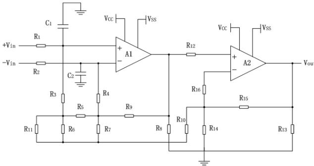
Fig. 6. AD626 Internal Connection
