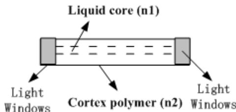
Fig. 3. Liquid-core optical fiber structures
