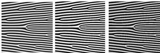
Fig. 4. (a) Holographic phase map with 256 levels, (b) its approximations with four equal steps, and (c) with four unequal steps
