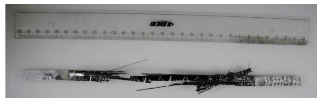
Fig. 3. Typical break in form of a brush of specimens cut from plate TKP2-1.
