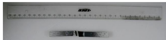
Fig. 9. Common failure of specimens cut along fibers direction from plate TKP1-4 subjected to compression tests.
