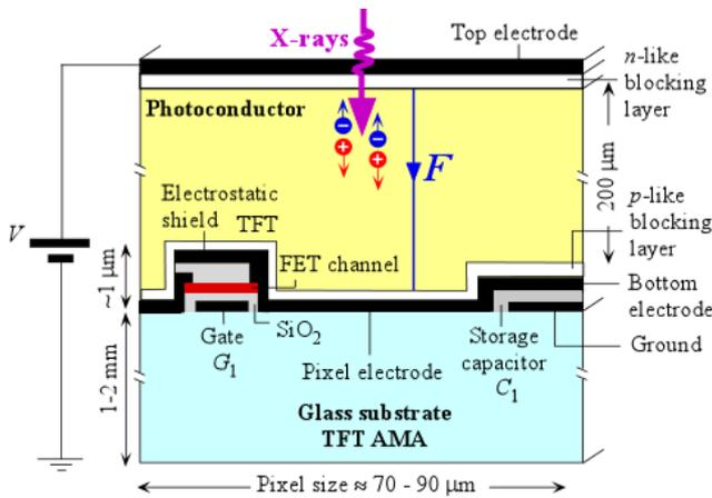
Fig. 8. A simplified schematic diagram of the cross section of a simple pixel with thin film transistor (TFT) [15].
