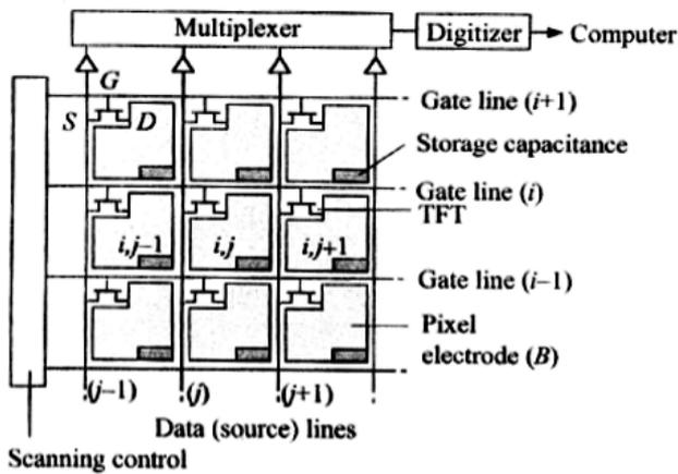
Fig. 7. A simplified schematic illustration of a FPXI and its peripheral electronics (see [15] for details & Ref's therein).
