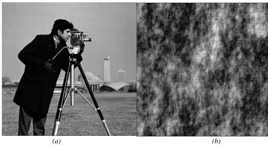
Fig. 1. (a) Grayscale cameraman image of size 256 x 256 pixels, (b) Fresnel transformed image ( \lambda = 632.8\text{nm} , propagation distance d_1 = 20\text{mm} and d_2 = 30\text{mm} )
