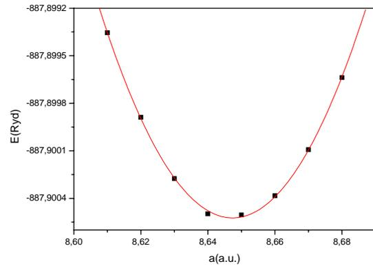
Fig. 2. Total energy as a function of the lattice constant for the monolayer c-BP/c-GaN bulk heterostructure.
