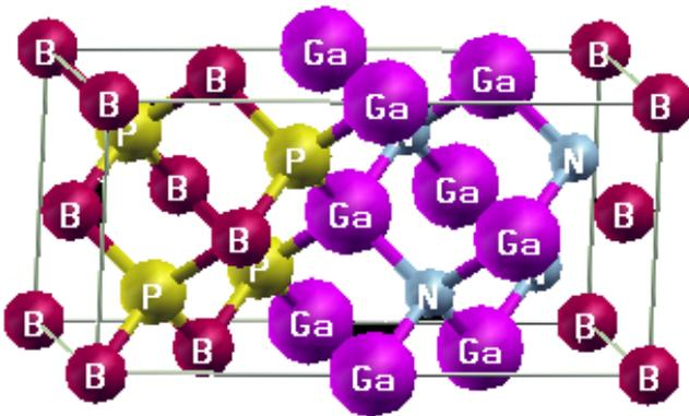
Fig. 1. Bulk heterostructure for c-BP/c-GaN system.
