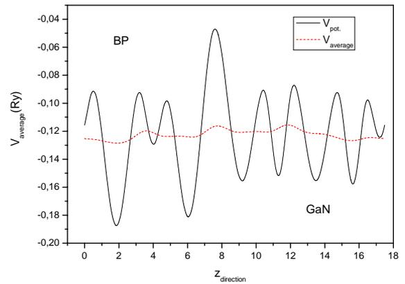
Fig. 3. Macroscopic average potential for c-BP/c-GaN bulk heterostructure.
