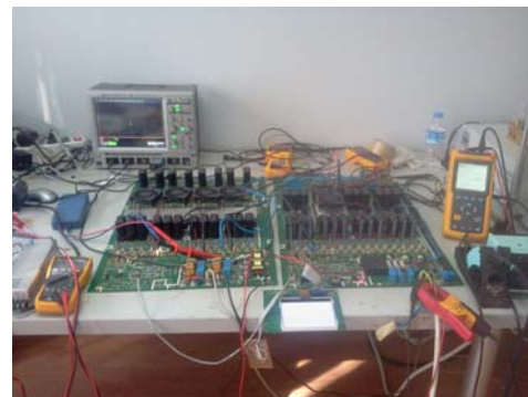
Fig. 6. Implementation of an MPPT Method which realizes the control and perturbations on the AC side.
