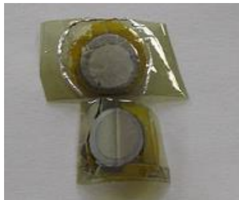
Fig. 11. Top view of the poly/ITO/CdS/CdTe photovoltaic cell.
