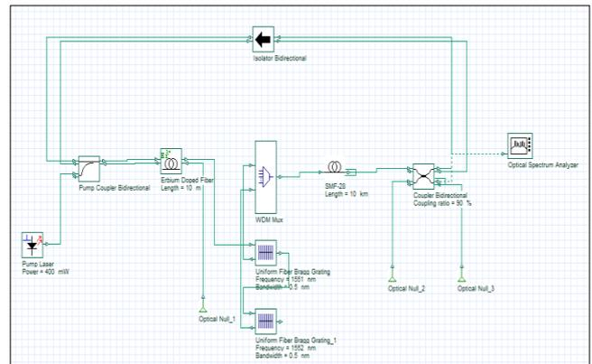
Fig. 4 Schematic design of EDFL system based on generation of four wave mixing (FWM) using software
