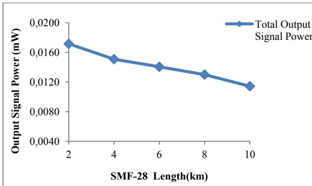
Fig. 9(b) Effect of SMF-28 length for system based on generation of FWM
