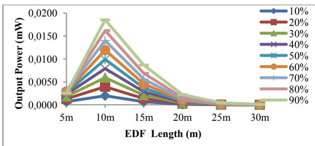
Fig. 6 Effect of EDF length for system based on two wavelengths
