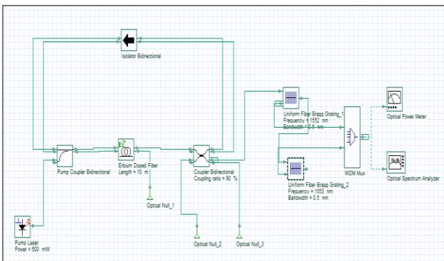
Fig. 2 Schematic design of EDFL system based on two wavelengths using software
