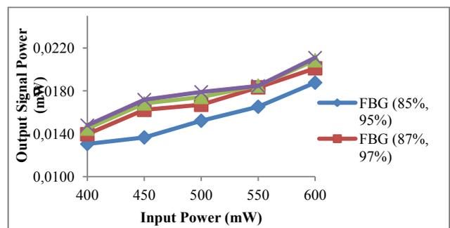
Fig. 8 Effect of different reflectivity combinations for input power of system based on two wavelengths
