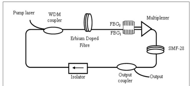
Fig. 3 Schematic design of EDFL system based on generation of four wave mixing (FWM)
