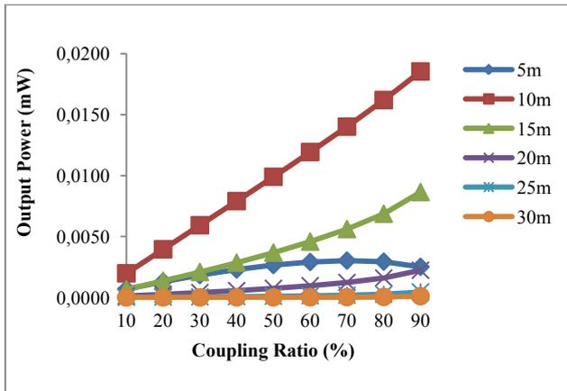
Fig. 5 Effect of coupling ratio for system based on two wavelengths
