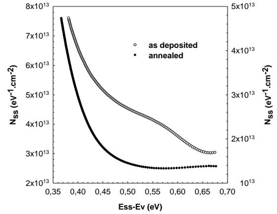
Fig. 3. Density of interface states  $N_{SS}$  as a function of  $E_{SS}-E_V$  deduced from the  $I-V$  data at room temperature.
