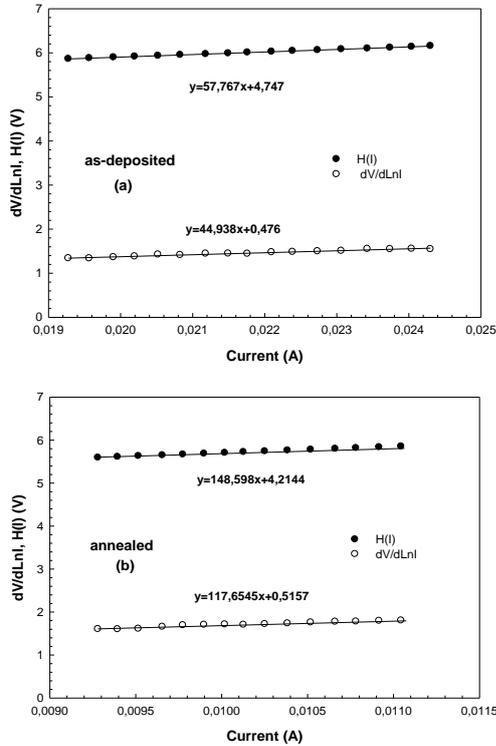
Fig. 2. The plots of  $dV/d\ln I$  and  $H(I)$  vs. current of Al/HfO<sub>2</sub>/p-Si(100) Schottky diode (a) as deposited and (b) annealed at 700 °C.
