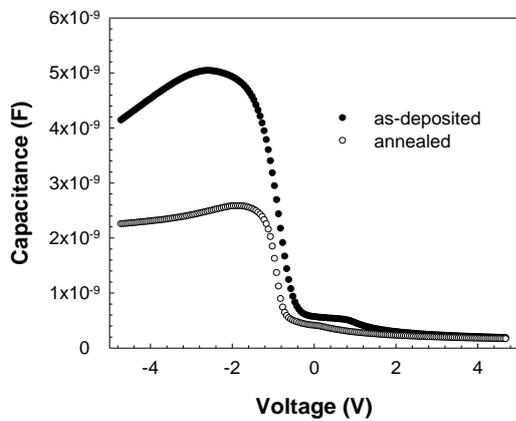
Fig. 4. Forward and reverse bias capacitance-voltage ( $C-V$ ) characteristics of the Al/HfO<sub>2</sub>/p-Si (100) Schottky diodes.
