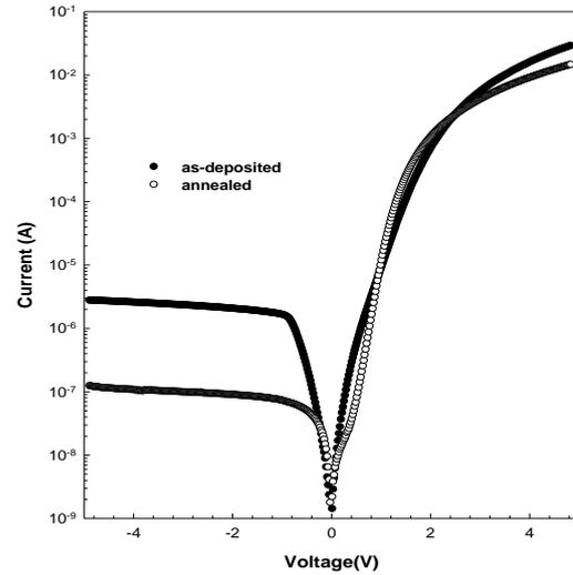
Fig. 1. Forward and reverse bias current-voltage ( $I$ - $V$ ) characteristics of the Al/HfO<sub>2</sub>/p-Si (100) Schottky diodes. "●" represents the data of the as-deposited sample and "○" represents the sample annealed at 700 °C.
