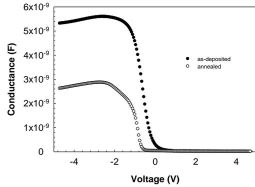
Fig. 5. Forward and reverse bias conductance-voltage ( $G/w-V$ ) characteristics of the Al/HfO<sub>2</sub>/p-Si (100) Schottky diodes.
