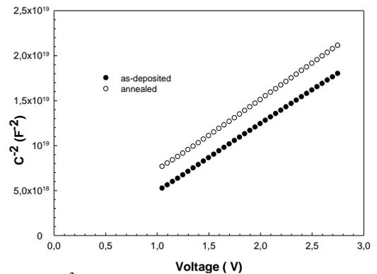
Fig. 6.  $C^{-2}-V$  characteristics of the Al/HfO<sub>2</sub>/p-Si (100) Schottky diodes.
