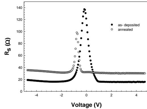
Fig. 7. The variation of the series resistance as a function of voltage at room temperature.
