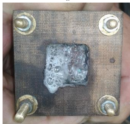
Fig.8. Copper plate assembly air pressure test: 2 bar (a) and 5 bar (b)
