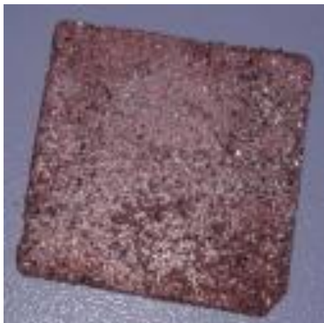
Fig. 6. Copper plate after the pressure test
