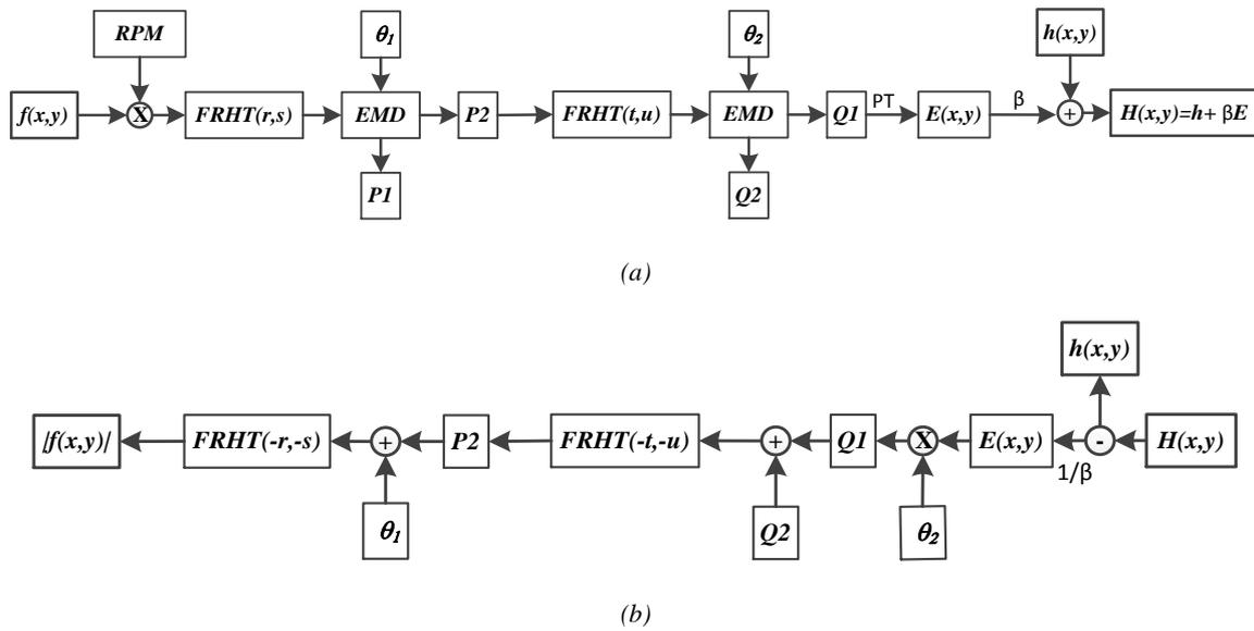
Fig. 5. Flowchart of encryption (a) and decryption scheme (b)
