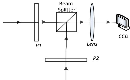
Fig. 3. Optical setup of the decryption process of the equal modulus decomposition
