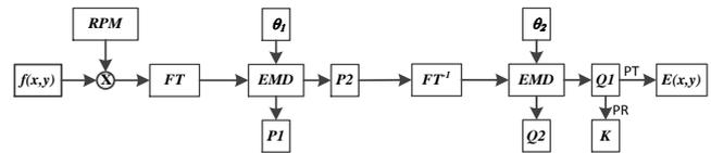
Fig. 4. Flowchart of the encryption scheme of modified equal modulus decomposition
