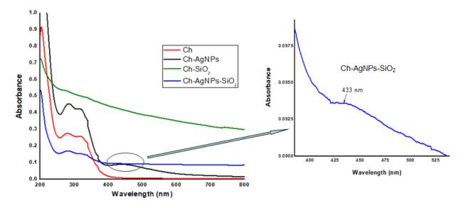
*Fig. 2. UV-Vis absorption spectra of the phyto-based materials. Inset: The spectral fingerprint of AgNPs (at 433 nm) in Ch-AgNPs-SiO<sub>2</sub> biohybrids (color online)*
