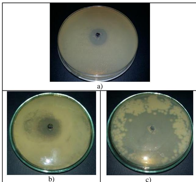
Fig. 4. Antibacterial efficiency of Ch-AgNPs (a) and of silica-based materials without (b) and with (c) Ch-AgNPs, towards *Escherichia coli* ATCC 8738 bacterium (color online)
