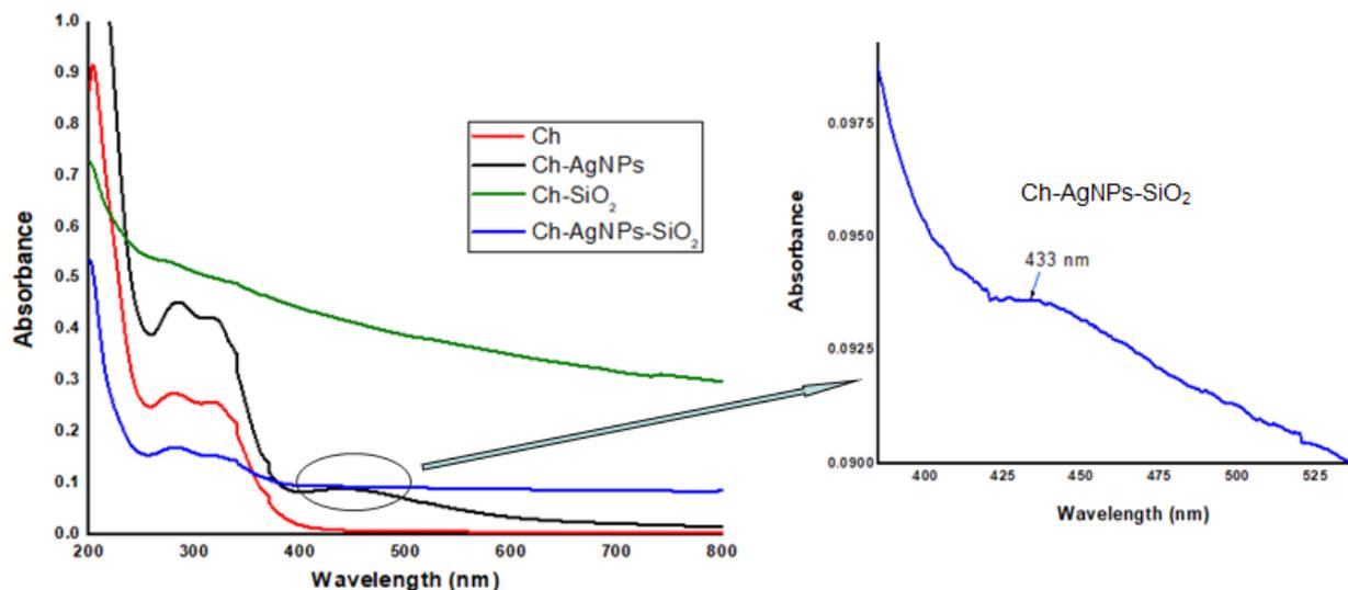
Fig. 2. UV-Vis absorption spectra of the phyto-based materials.
