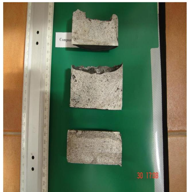
Fig. 4. Macrography of the three types of cellular composite studied for achieving modeling and fractal analysis
