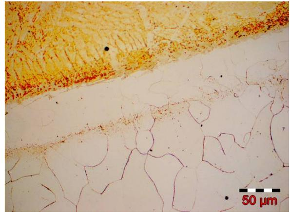
Fig. 7.b. Fusion line with elemental accumulation, due to heat treatment at 900°C for 6 hours.
