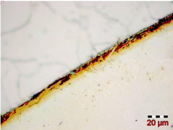
Fig. 5.b. Fusion line with elemental accumulation due to heat treatment at 600°C for 4 hours.
