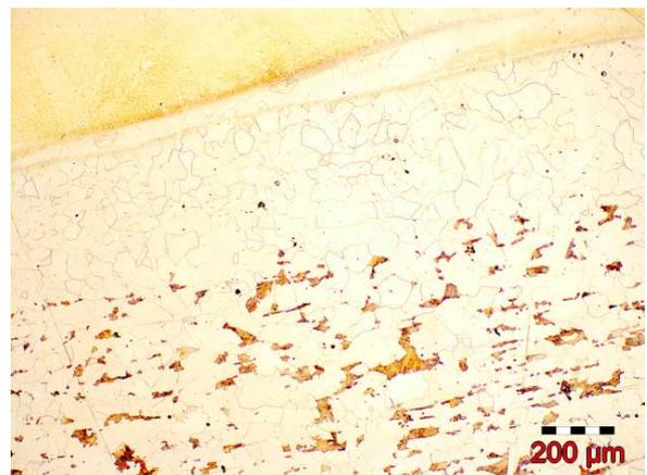
Fig. 8. Heat affected zone for heat treated sample at 900°C/6 hours/furnace cooled.
