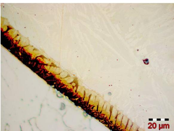
Fig. 6.b. Fusion line with elemental accumulation, due to heat treatment at 600°C for 6 hours.
