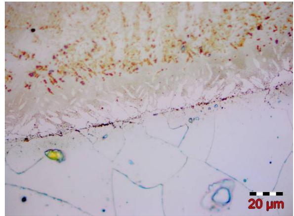
Fig. 7.a. Fusion line with elemental accumulation, due to heat treatment at 900°C for 6 hours.
