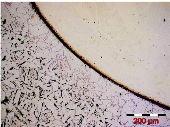
Fig. 6.a. Fusion line with elemental accumulation, due to heat treatment at 600°C for 6 hours.
