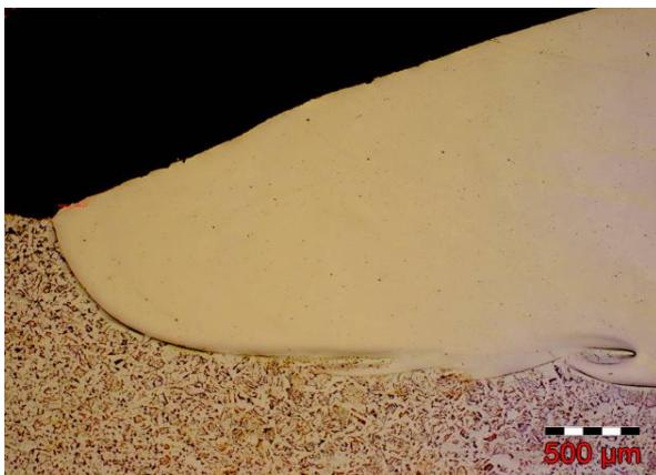
Fig. 4.a. Macroscopic appearance of weld deposit with high entropy alloy before applying heat treatment (x50).
