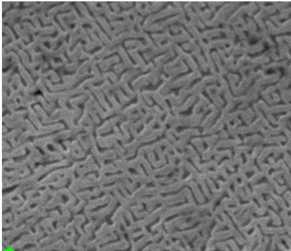
Fig. 3. High entropy alloy microstructure. SEM microscopy. (x10000).
