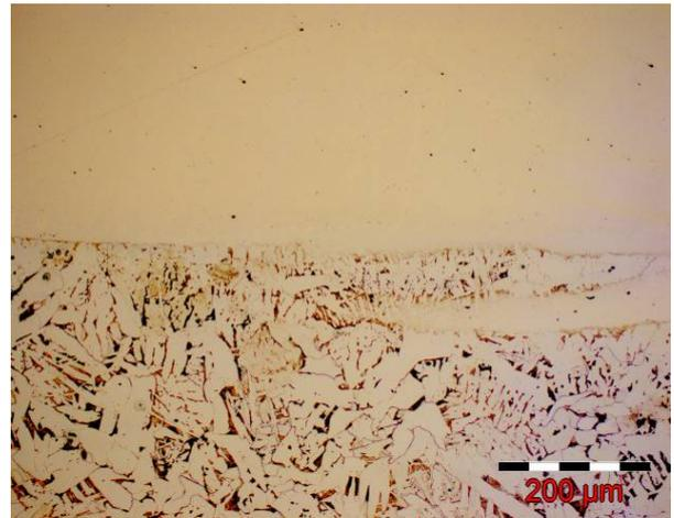
Fig. 4.b. Macroscopic appearance of weld deposit with high entropy alloy before applying heat treatment (x100).
