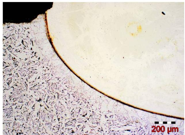
Fig. 5.a. Fusion line with elemental accumulation due to heat treatment at 600°C for 4 hours.
