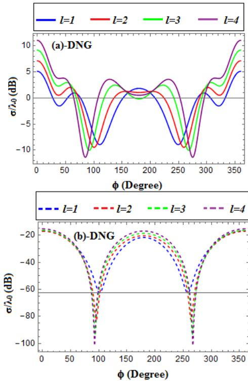
Fig. 6. The influence of the OAM mode index ( $l$ ) on the normalized bistatic echo width under TE polarization for DNG-coated metamaterial: (a) co-polarized field component and (b) cross-polarized field component (color online)
