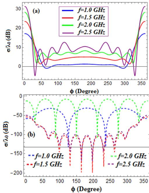
Fig. 7. The influence of beam frequency on the normalized bistatic echo width for  $a = 5$  cm,  $b = 10$  cm: (a) co-polarized field component and (b) cross-polarized field component (color online)
