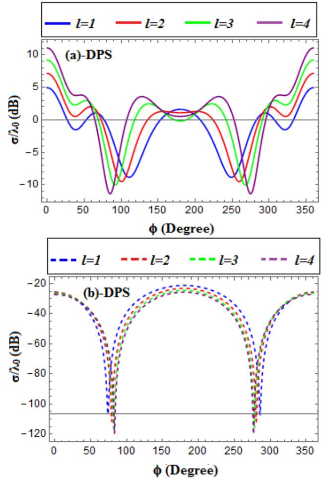
Fig. 5. The influence of the OAM mode index ( $l$ ) on the normalized bistatic echo width under TE polarization for DPS-coated metamaterial: (a) co-polarized field component and (b) cross-polarized field component (color online)
