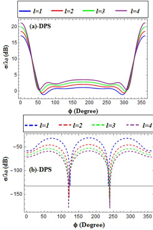
Fig. 3. The influence of the OAM mode index ( $l$ ) on the normalized bistatic echo width under TM polarization for DPS-coated metamaterial: (a) co-polarized field component and (b) cross-polarized field component (color online)
