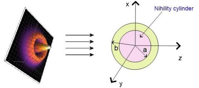
Fig. 1. The nihility coated cylinder illuminated by an LG beam (color online)
