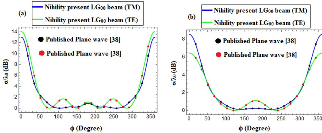
Fig. 2 Graphical comparison between TM and TE scattering field coefficients of the nihility cylinder coated with metamaterials ( $f = 1$  GHz,  $a = 5$  cm,  $b = 10$  cm,  $\epsilon_{r1} = \pm 9.8$ , and  $\mu_{r1} = \pm 1$ ) (a) DPS (b) DNG (color online)
