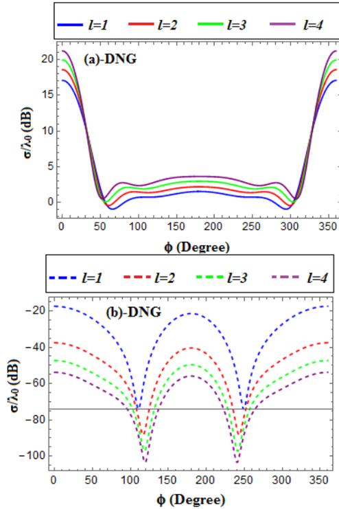
Fig. 4. The influence of the OAM mode index ( $l$ ) on the normalized bistatic echo width under TM polarization for DNG-coated metamaterial: (a) co-polarized field component and (b) cross-polarized field component (color online)
