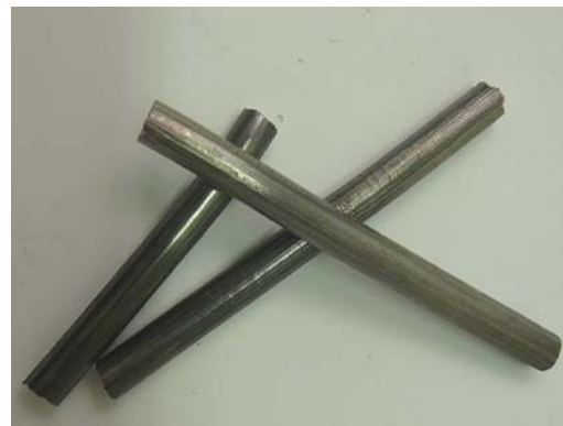
Fig.3. Micrographic aspect of the Al-2%vol. \text{Al}_2\text{O}_3 extruded bars.
