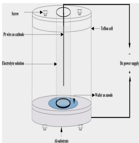
Fig. 1. Schematic of the designed porous silicon fabrication system.
