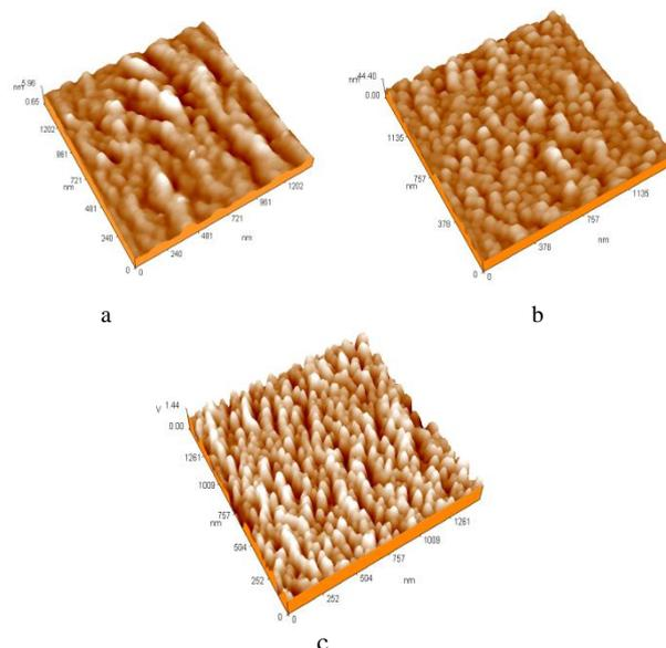
Fig. 2. 3D AFM images of the nanostructures porous silicon samples with etching time (a) 10 min (b) 20 min and (c) 30 min.
