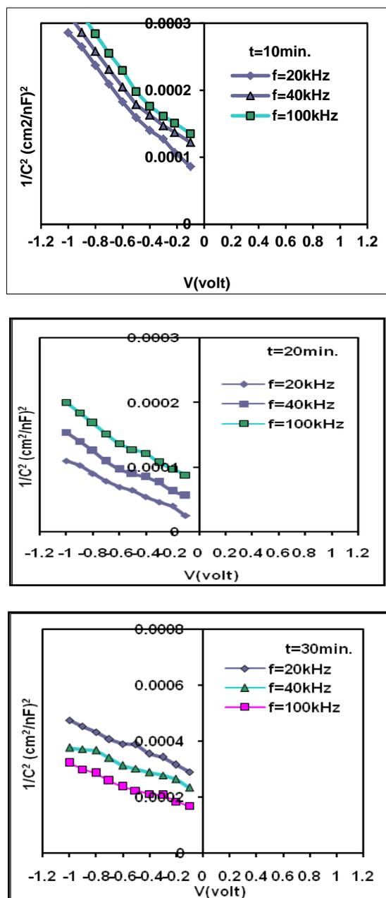
Fig. 5. The capacitance-Voltage characteristics of Au/PS/p-Si/Al which prepared at fixed current density of 50 mA/cm<sup>2</sup> and different etching time (a) 10 min (b)20min. (c) 30min and different frequencies.
