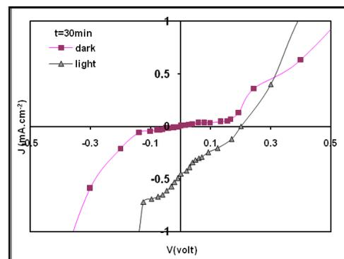
Fig. 4. The J-V characteristics of (Au/PS/p-Si/Al) at different etching time: (a) 10 min (b) 20 min (c) 30 min.
