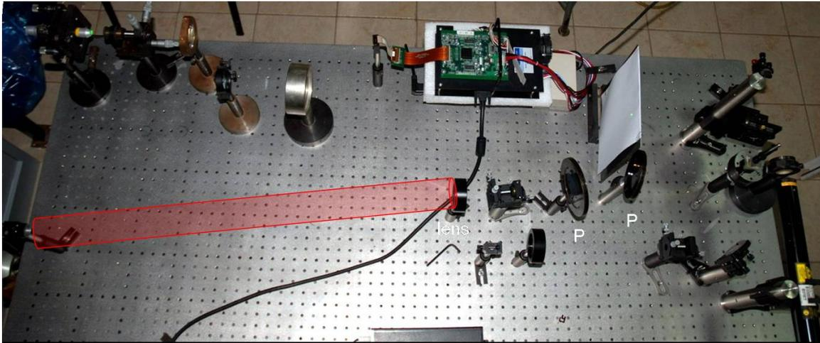
Fig. 3. The experimental arrangement for Fresnel holography. The only notable difference in this arrangement compared to Fig. 1 is that the reference is a plane wave instead of spherical wave.
