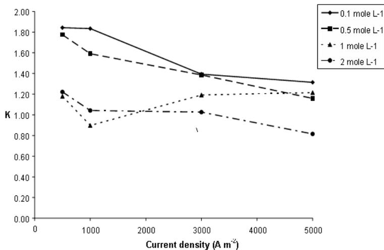
Fig. 7. The dependence of  $K$  on the applied current density for a polarity reversal period of 4 minutes.
