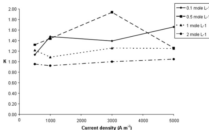
Fig. 4. The dependence of  $K$  on the applied current density for a polarity reversal period of 1 minute
