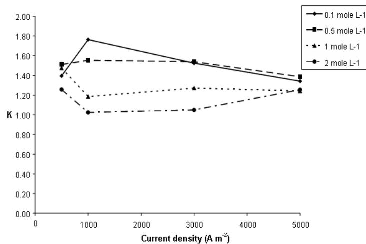
Fig. 6. The dependence of  $K$  on the applied current density for a polarity reversal period of 3 minutes.
