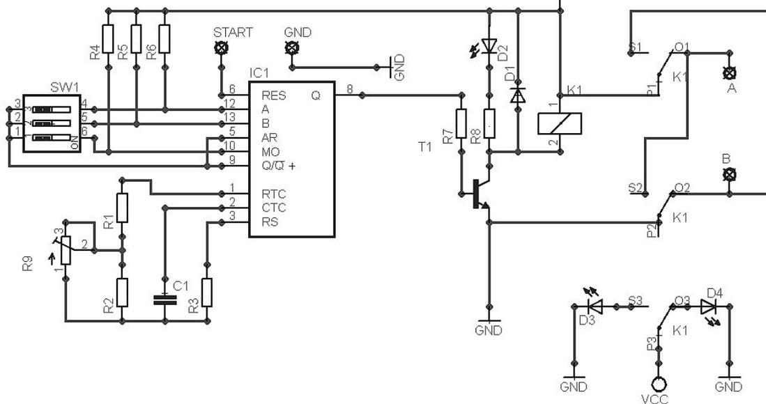
Fig. 2. Depiction of the electronic scheme of CD4541 timer adapted using a basic timer scheme [30]
