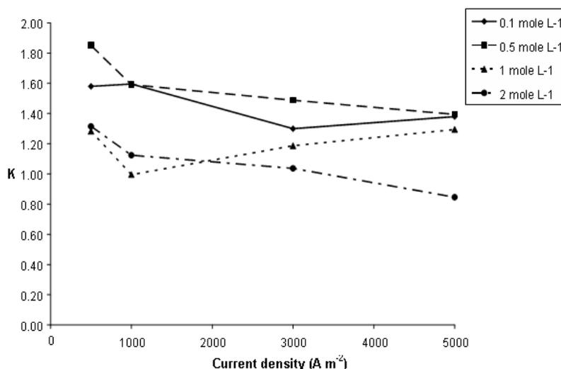
Fig. 8. The dependence of  $K$  on the applied current density for a polarity reversal period of 5 minutes.
