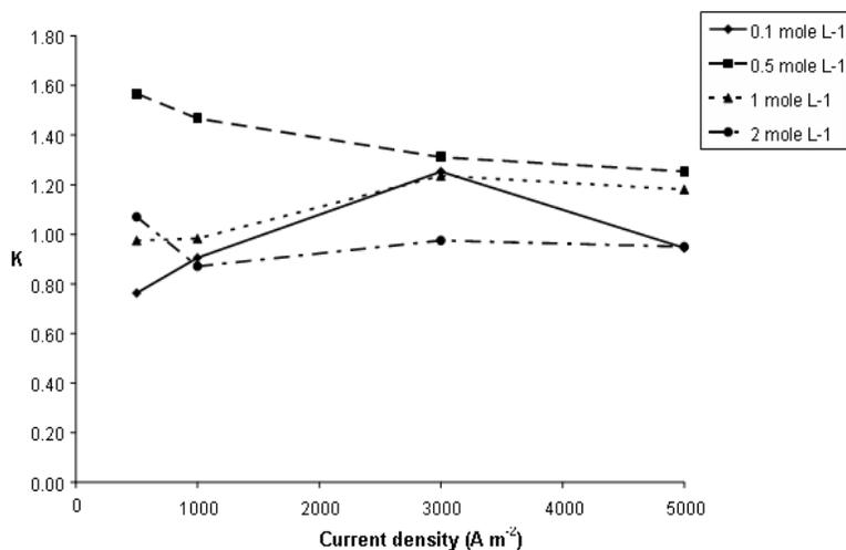
Fig. 9. The dependence of  $K$  on the applied current density for a polarity reversal period of 10 minutes.
