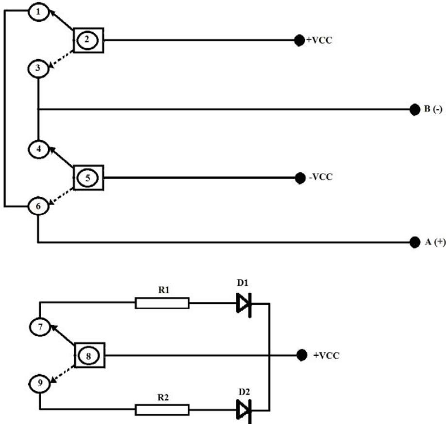
Fig. 3. A depiction of the relays connecting scheme of the polarity reversal device
