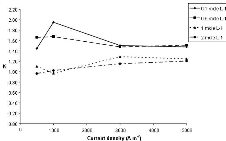
Fig. 5. The dependence of  $K$  on the applied current density for a polarity reversal period of 2 minutes.
