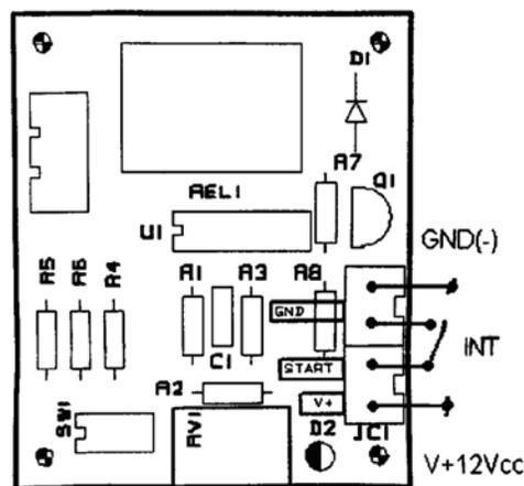
Fig. 1. The printed circuit board layout of the CD4541 electronic timer [30].
