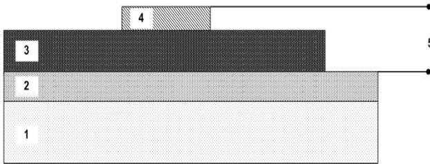
Fig.4. Schematic diagram of the CuPc and H<sub>2</sub>Pc bulk heterojunction sample: glass substrate (1), conductive glass (2), CuPc-H<sub>2</sub>Pc thin film (3), aluminium film (4), terminals (5).
