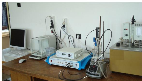
Fig.1 Voltalab 10 equipment for electrodeposition and corrosion measurements
