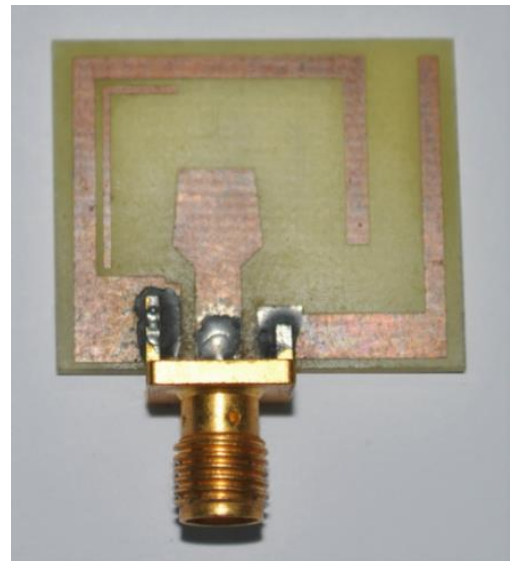
Fig. 6. A photograph of the fabricated antenna (color online)
