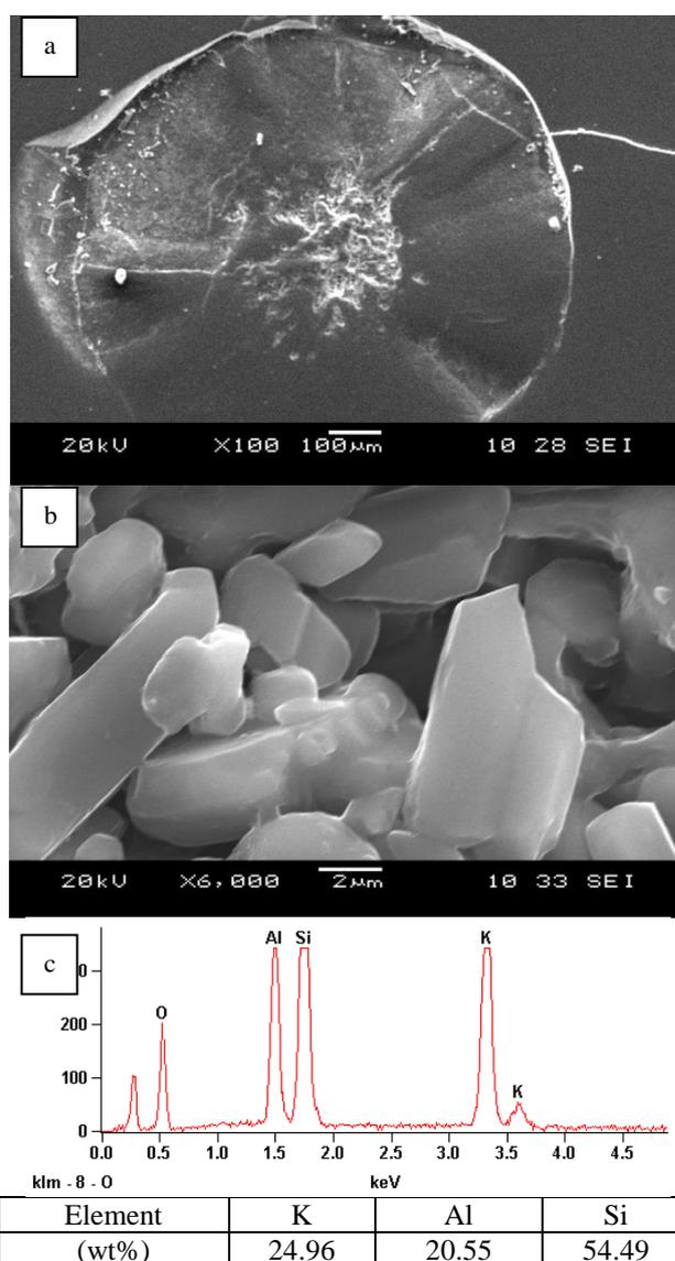
Fig. 2. SEM images at lower (a) and higher (b) magnifications and EDS elemental analysis (c) of the crystals shown in the image (b)
