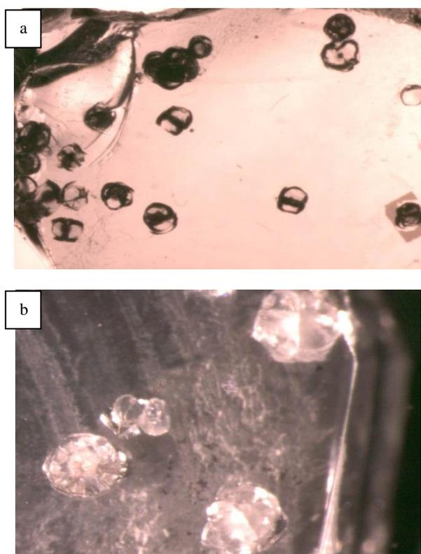
Fig. 1. Images of sections of the glass, containing leucite crystals, at lower (a) and higher (b) magnifications, obtained with stereo-optical microscope (for scale estimation, the bigger crystals are about 250 - 300  $\mu\text{m}$ )
