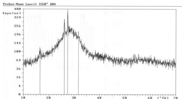
Fig. 3. The X-ray diffractogram confirms that leucite crystals have been crystallized in the glass matrix. (Leucite PDF card 38-1423)
