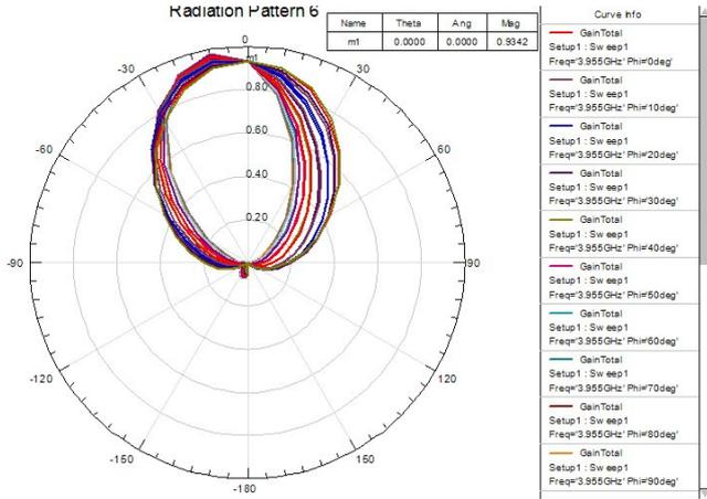
Fig. 12. Radiation pattern for DRA coupled to a 48 mm microstrip line by a 7mm on 2mm slot at 3,955GHz
