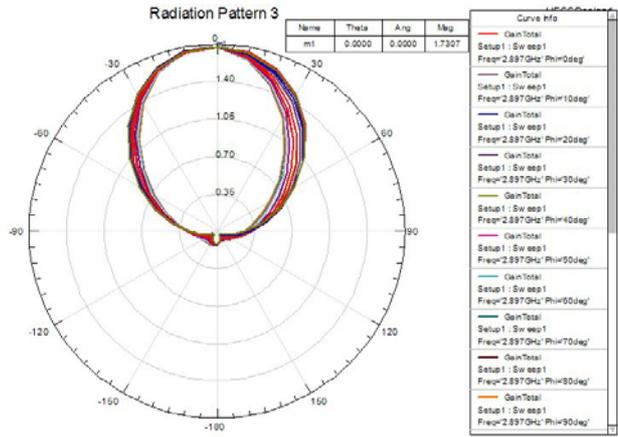
Fig. 6. Radiation pattern of the DRA fed by a slot 6mm, on 1mm, from a 40 mm length microstrip at 2.897GHz
