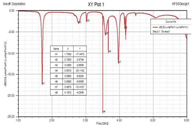
Fig. 14 The simulated return loss for the DRA coupled to a 48mm microstrip line by a 7mm on 2mm slot and with an air gap of  $S_{11}$  10µm
