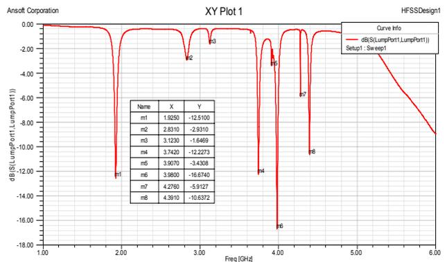
Fig. 16 The simulated return loss for the DRA coupled to a 48mm microstrip line by a 7mm on 2mm slot and with an air gap of  $S_{11}$  50µm [6]
