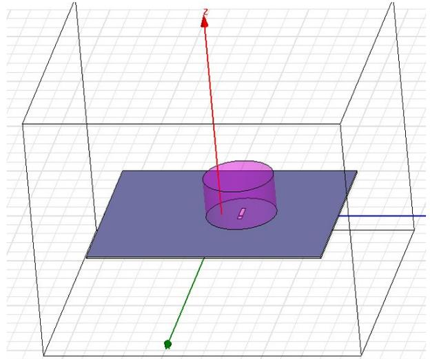
Fig. 1 Cylindrical resonator antenna fed by a slot coupled microstrip line.
