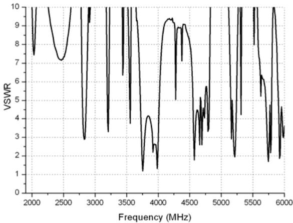
Fig. 13 The measured voltage standing wave ratio (VSWR) for the DRA coupled to a 48 mm microstrip line by a 7mm on 2mm slot
