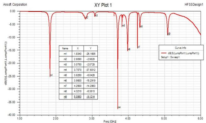
Fig. 15 The simulated return loss for the DRA coupled to a 48mm microstrip line by a 7mm on 2mm slot and with an air gap of  $S_{11}$  30µm.
