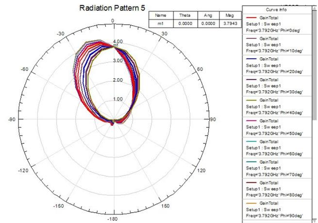
Fig.11. Radiation pattern for DRA coupled to a 48 mm microstrip line by a 7 mm on 2 mm slot at 3,792GHz
