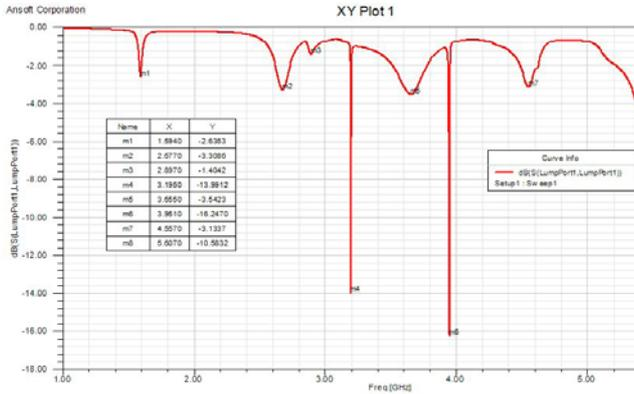
Fig. 3 The return loss for a cylindrical DRA coupled to a 40 mm microstrip line with a 6 mm by 1 mm slot.
