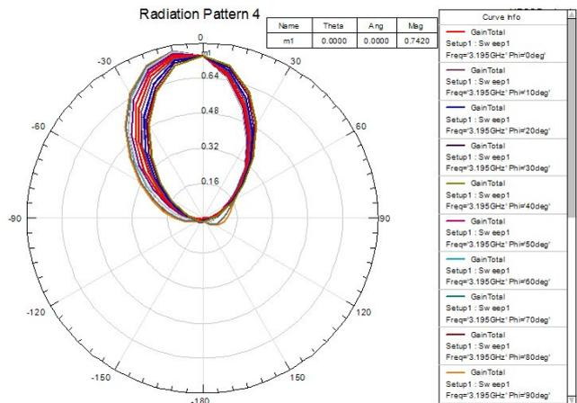
Fig.7. Radiation pattern of the DRA fed by a slot 6mm, on 1mm, from a 40 mm length microstrip at 3.195GHz
