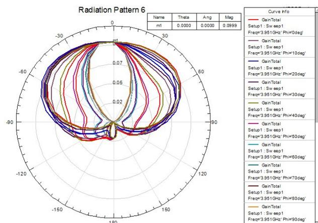
Fig. 9. Radiation pattern of the DRA fed by a slot 6mm, on 1mm, from a 40 mm length microstrip at 3,951 GHz
