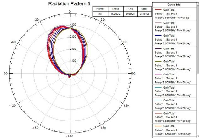
Fig. 8. Radiation pattern of the DRA fed by a slot 6mm, on 1mm, from a 40 mm length microstrip at 3,655GHz
