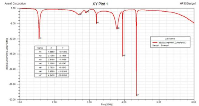
Fig. 10 The simulated return loss for the DRA coupled to a 48mm microstrip line by a 7mm on 2mm slot.
