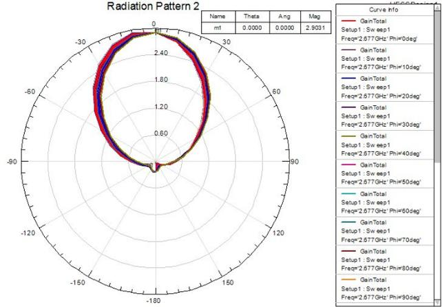
Fig. 5. Radiation pattern of the DRA fed by a slot 6mm, on 1mm, from a 40 mm length microstrip at 2.677GHz
