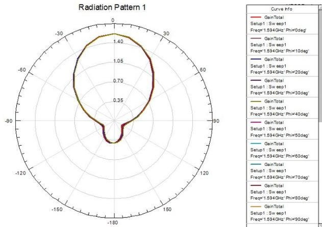
Fig. 4. Radiation pattern of the DRA fed by a slot 6mm, on 1mm, from a 40 mm length microstrip at 1.594GHz
