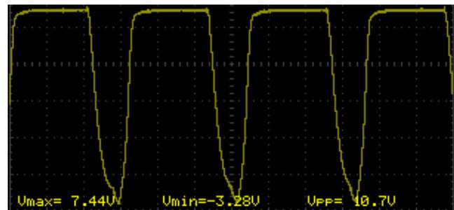
Fig. 9. Received audio signal after being amplified
