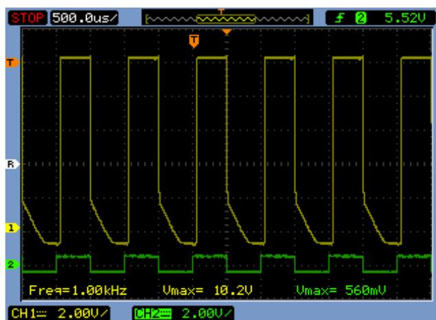
Fig. 8. The 1 kHz signal before and after amplification
