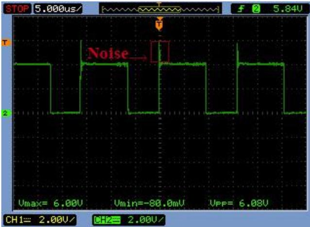
Fig. 10. Transmitted signal and effect of the system internal noise
