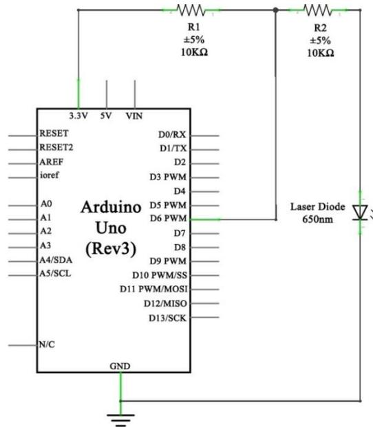
Fig. 16. Transmitter circuit diagram
