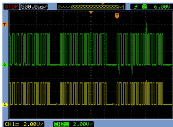
Fig. 21. Transmitted and received text signals
