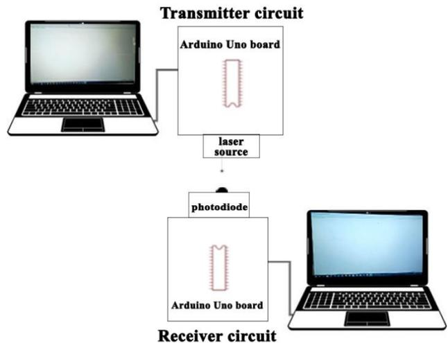
Fig.15. Text transmission implemented model diagram
