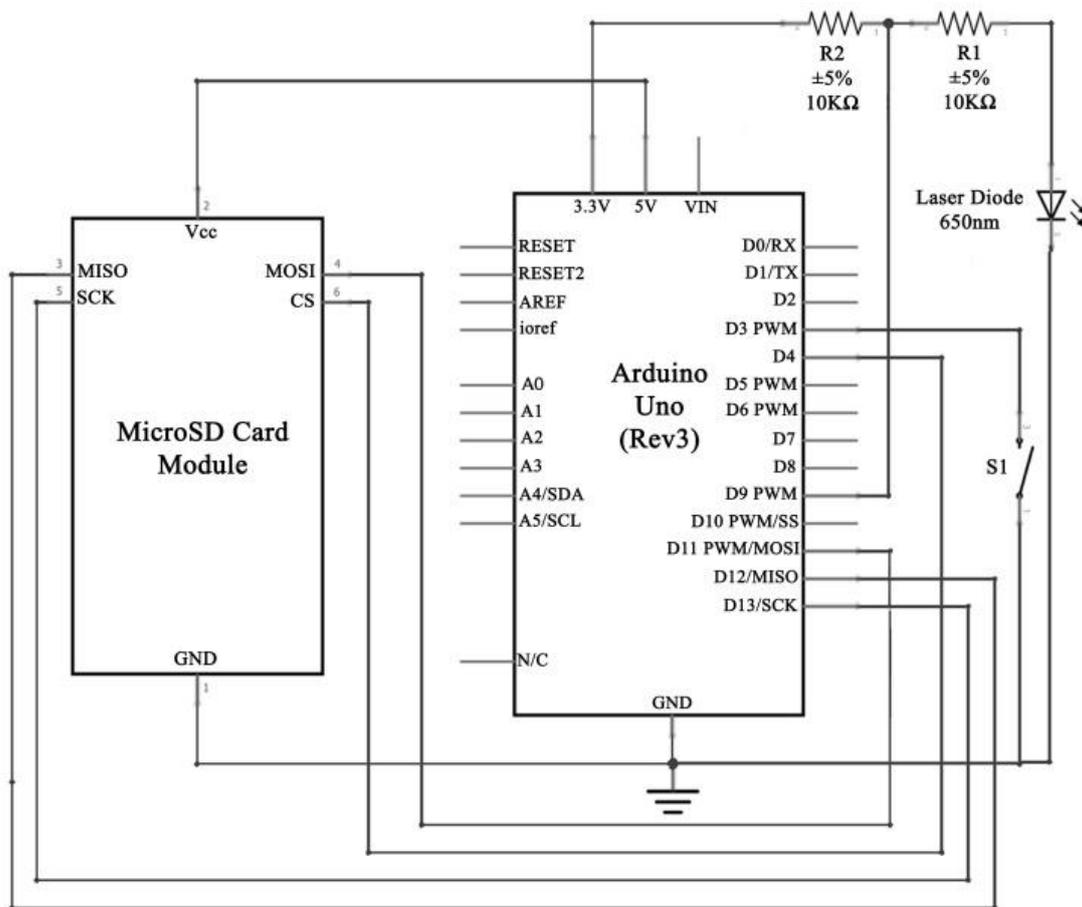
Fig. 2. Transmitter circuit design
