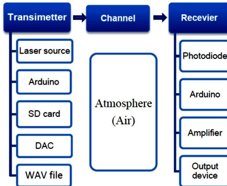
Fig. 1 Audio system configuration
