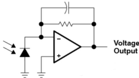
Fig. 5. TSL250R functional block diagram [8]
