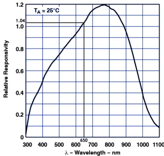
Fig. 6. TSL250R photodiode spectral responsivity [8]
