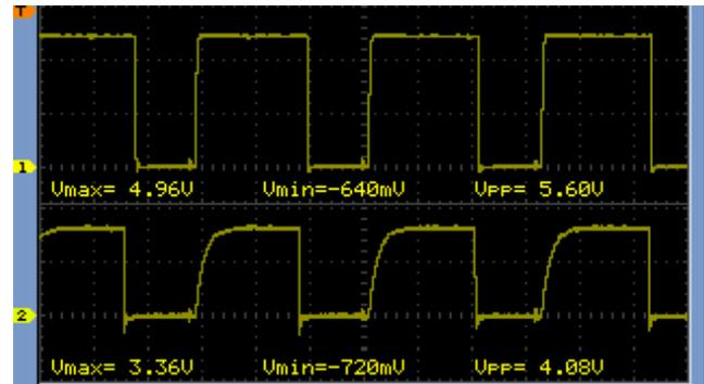
Fig. 11. Comparison between the received signals using the Arduino (1) vs. not using the Arduino (2)
