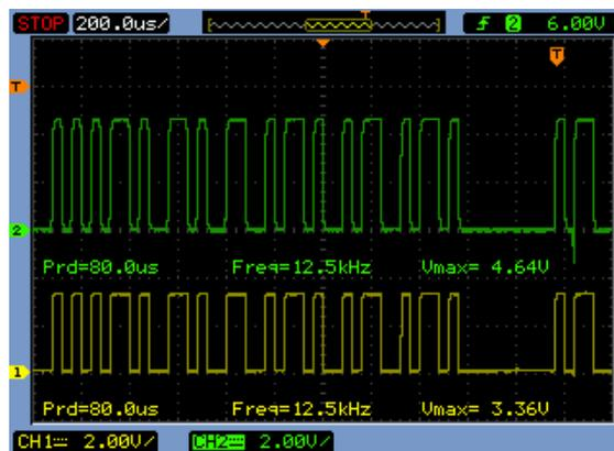
Fig. 20. Transmitted and received text signals
