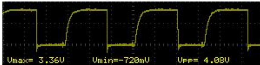
Fig. 7. The received signal after the photodiode circuit
