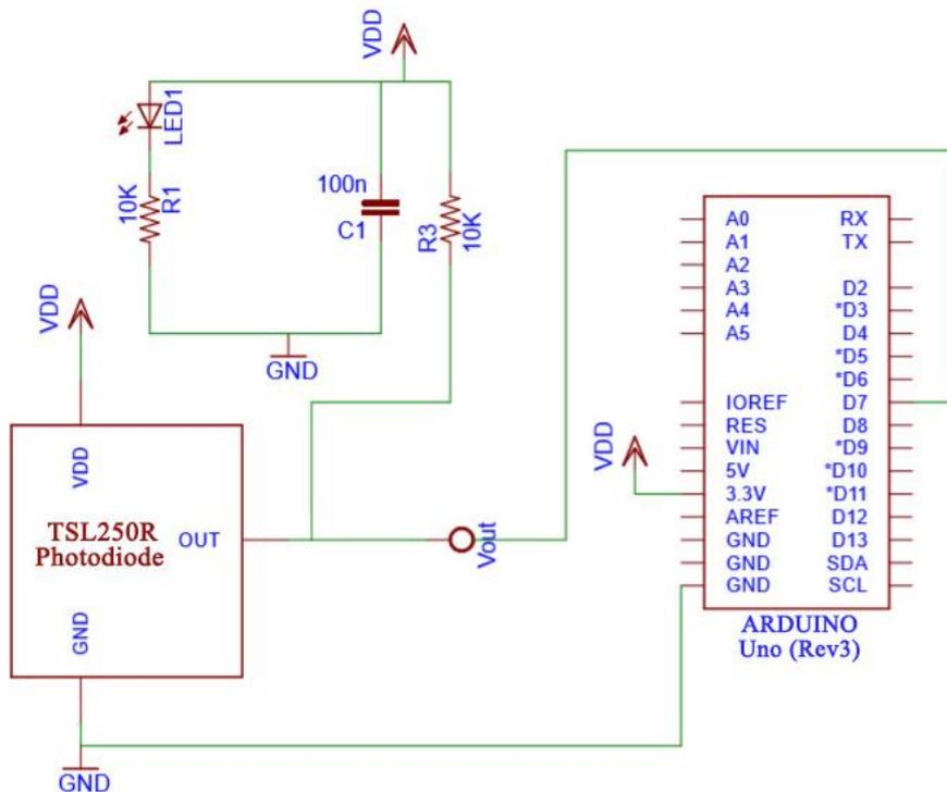
Fig. 17. The receiver circuit design diagram
