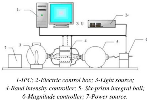
Fig. 1. The structure of the new single star simulator.
