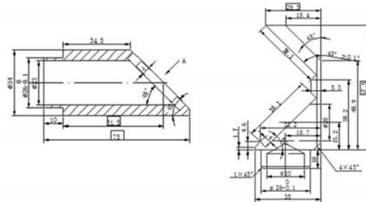
Fig. 6. The assembly diagram of the mirror groups.
