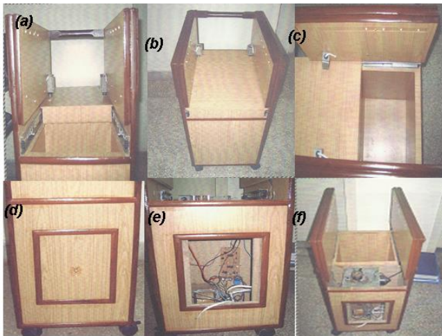
Fig. 4. (a) Shielding with open lid and sensors; (b) shielding with closed lid and wooden handle; (c) Top view with sensors and limit switches; (d) Back view of shielding; (e) Electrical Panel; (f) division of main shielding box.
