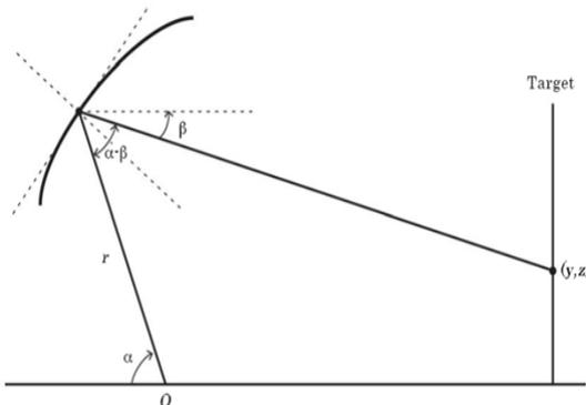
Fig.4. 2-D reflector profile structure for a near-field problem using detailed numerical integration method by Elmer [9].
