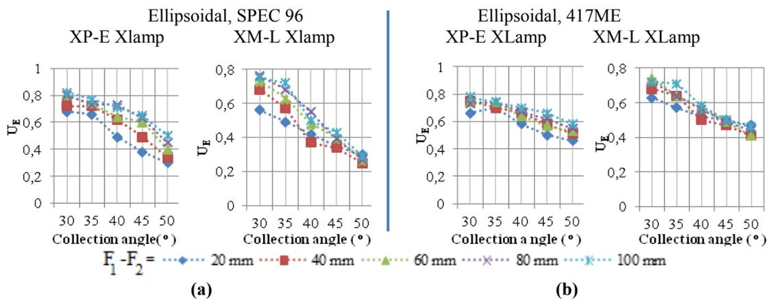
Fig.8. Uniform lighting values of ellipsoidal reflectors with 30°,35°,40°,45°,50° collection angles, and 20, 40, 60, 80, 100mm distance between two focal points for XP-E Xlamp and XM-L Xlamp power LEDs (a) 88% specular reflectance (b) 88% semi-specular reflectance
