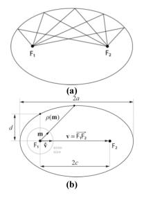
Fig. 1 (a) When a light source is placed on a focal point  $(F_l)$ , all lights travel on the other focal point  $(F_2)$  (b) Parameters of ellipsoidal on polar coordinates.
