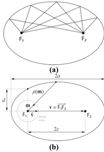
Fig. 1 (a) When a light source is placed on a focal point ( $F_1$ ), all lights travel on the other focal point ( $F_2$ ) (b) Parameters of ellipsoidal on polar coordinates.
