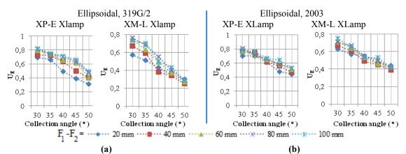
Fig.7. Uniform lighting values of ellipsoidal reflectors with 30°,35°,40°,45°,50° collection angles, and 20, 40, 60, 80, 100mm distance between two focal points for XP-E Xlamp and XM-L Xlamp power LEDs (a) 88% specular reflectance (b) 88% semi-specular reflectance
