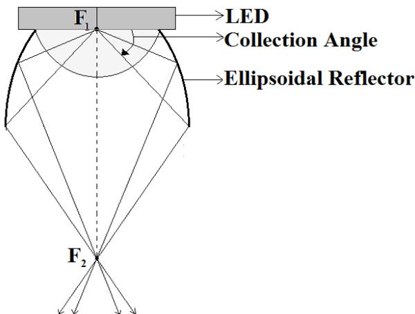
Fig.2. Ellipsoidal reflector obtained with LED source.
