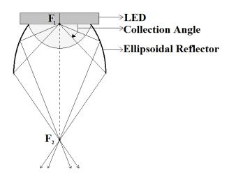
Fig.2. Ellipsoidal reflector obtained with LED source.
