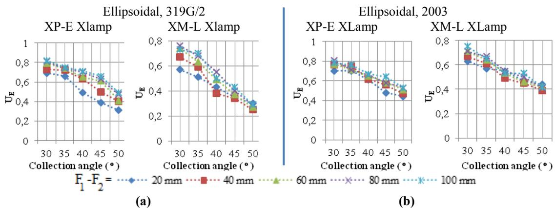
Fig.7. Uniform lighting values of ellipsoidal reflectors with 30°,35°,40°,45°,50° collection angles, and 20, 40, 60, 80, 100mm distance between two focal points for XP-E Xlamp and XM-L Xlamp power LEDs (a) 88% specular reflectance (b) 88% semi-specular reflectance
