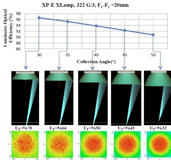
Fig. 5 Examples for the effect of ellipsoidal reflector designed with 20 mm distance between two focal points, and XP-E Xlamp LED lamp, when coated with 85 % reflectance specular reflector material on luminaire optical efficiency according to collection angles. With these values, uniformity values of lighting were given and denoted with arrows.
