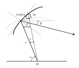
Fig.3. 2-Dimensional reflector profile structure for a farfield problem using detailed numerical integration method by Elmer [10].
