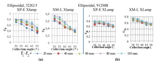
Fig.6. Uniform lighting values of ellipsoidal reflectors with 30°,35°,40°,45°,50° collection angles, and 20, 40, 60, 80, 100 mm distance between two focal points for XP-E Xlamp and XM-L Xlamp power LEDs (a) 85 % specular reflectance (b) 85 % semi-specular reflectance
