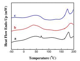
Fig. 3. DSC thermograms (10 °C/min) of (a) O-BAT-PU, (b) E-BAT-PU, and (c) U-BAT-PU.
