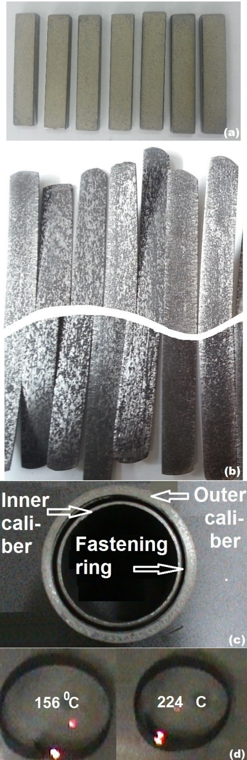
Fig. 4. Processing flow of FeMnSiCrNi PM specimens: (a) sintered specimens; (b) hot rolled specimens; (c) ring-shape setting with calibres; (d) training stages
