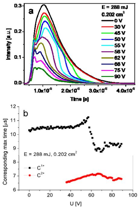
Fig. 3. Electrostatic energy analyzer in RFA mode: (a) TOF signals and (b) corresponding maximum time for  $C^{2+}$  and  $C^{1+}$  as a function of retarding voltage.
