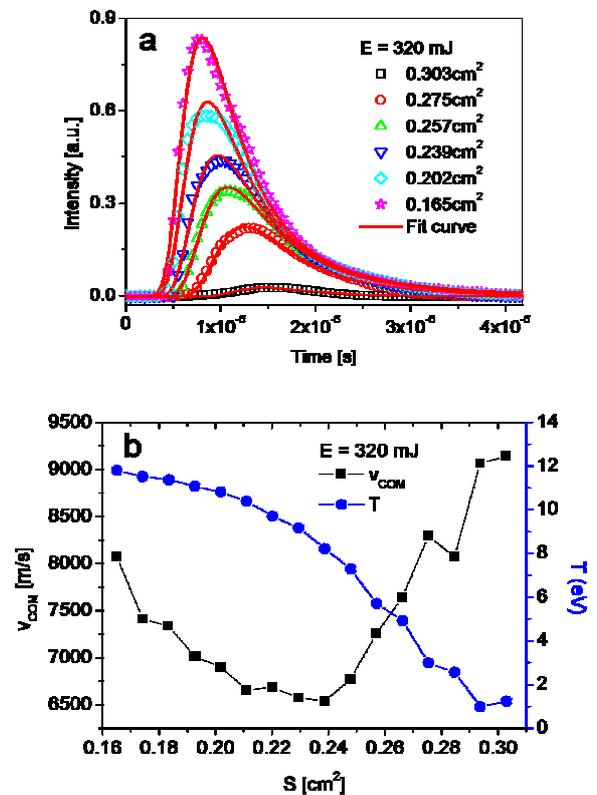
Fig. 2. Electrostatic energy analyzer in TOF mode: (a) TOF spectra and (b) derived temperature and  $v_{\text{COM}}$  variation for different laser spot size.
