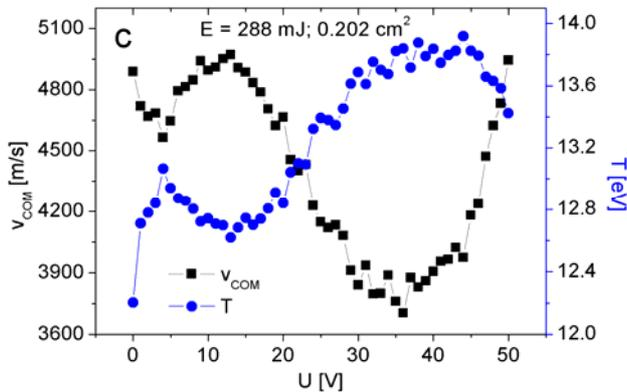
Fig. 4. Temperature and centre of mass velocity variation as a function of retarding voltage.
