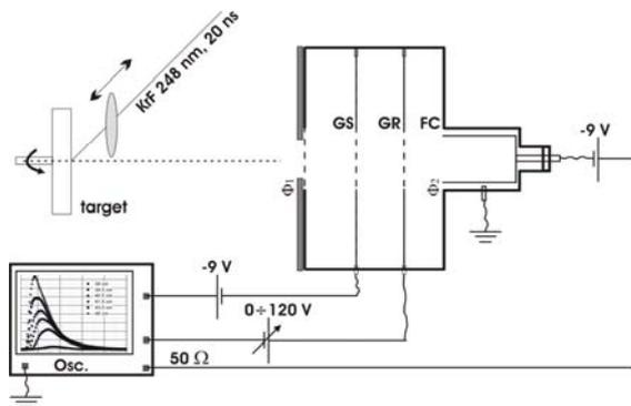
Fig. 1. Experimental set-up scheme (the bias voltage for GS and FC were assured by 9 V electric batteries in order to avoid unwanted electrical signal influences).
