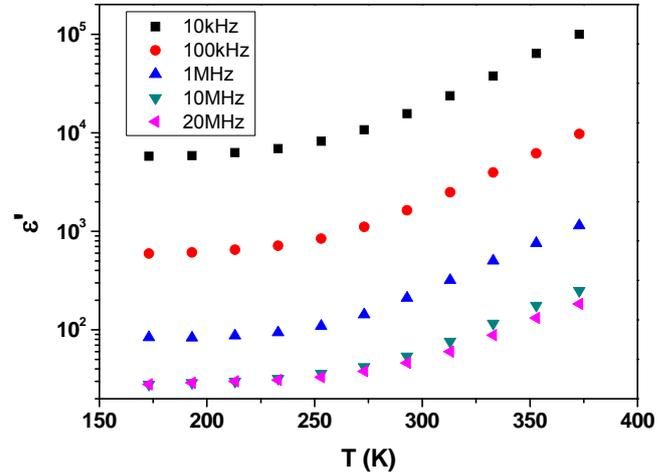
Fig. 6. Variation of the dielectric loss with temperatures at different frequencies
