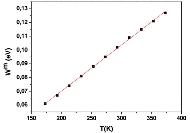
Fig. 7. Temperature dependence of the maximum barrier height
