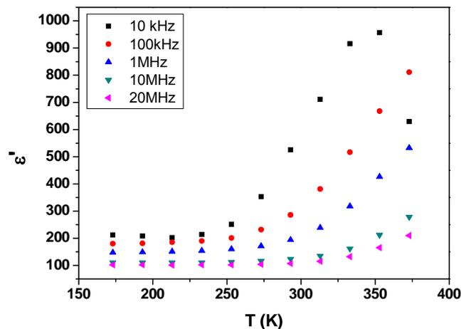
Fig. 4. Variation of the dielectric constant with temperatures at different frequencies
