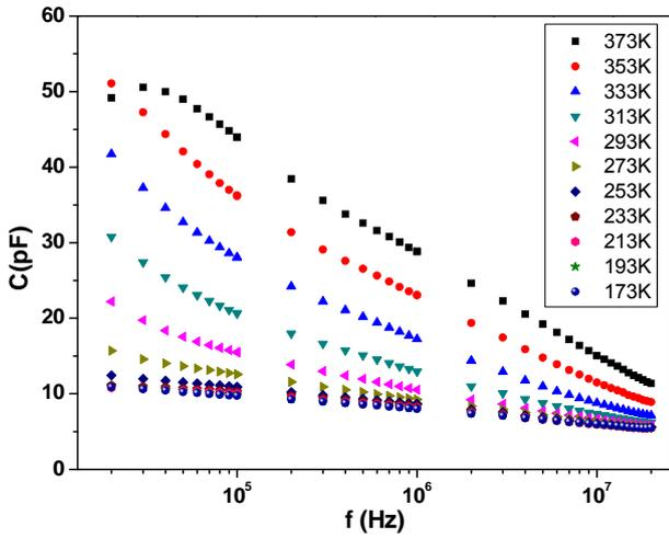
Fig. 1. Frequency dependence of capacitance at different temperatures
