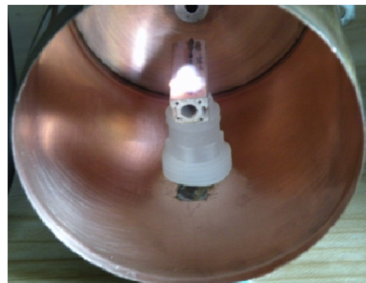
Fig. 4 Two lead wires are vaporized and ionized at 150W microwave power
