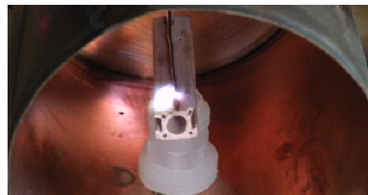
Fig. 3 The zinc sample is vaporized and ionized at 150W microwave power
