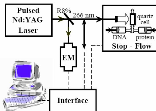
**Fig. 2.** Experimental set-up for high-resolution UV laser induced dynamic DNA – protein footprinting.
