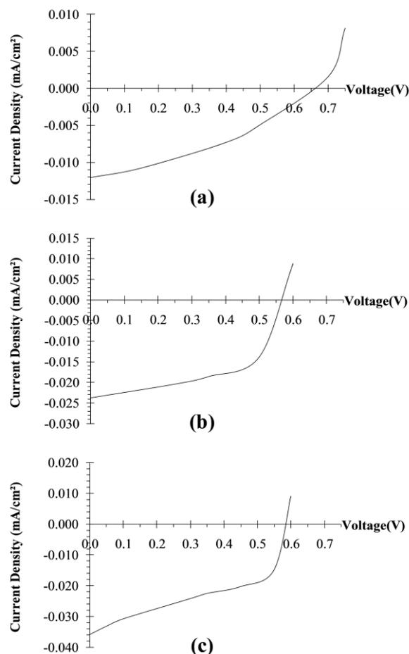
Fig. 7. J-V Curves of the fabricated solar cells using BTD with different weight ratios of (a) 0, (b) 5 and (c) 20 wt % showing threefold increase on the output power and  $J_{sc}$  and no noticeable change in the  $V_{oc}$
