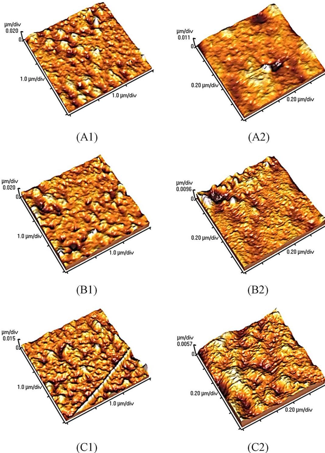
Fig. 6. The AFM height images of the solar cells active layer using BTB with different weight ratios of (a) 0, (b) 5 and (c) 20 wt % in two sizes ( $3 \times 3$  and  $1 \times 1 \mu\text{m}^2$ ) indicating that the surface roughness of the solar cell active layer decreases with increase in BTB weight ratio
