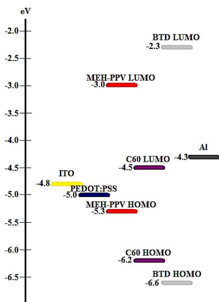
Fig. 5. Energy diagram of the fabricated solar cells showing high energy difference between BTD HOMO/LUMO and other materials energy levels
