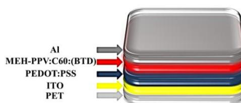
Fig. 1. The structure of the fabricated solar cells comprised of inactive PET substrate, ITO anode electrode, PEDOT:PSS buffer layer, MEH-PPV: $C_{60}$  (2:1) BTD active layer and Al cathode electrode
