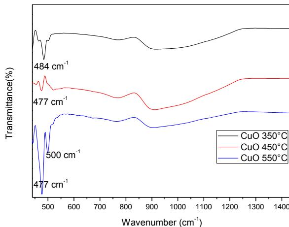
Fig.3. FTIR spectra of CuO thin films at different Annealing temperatures
