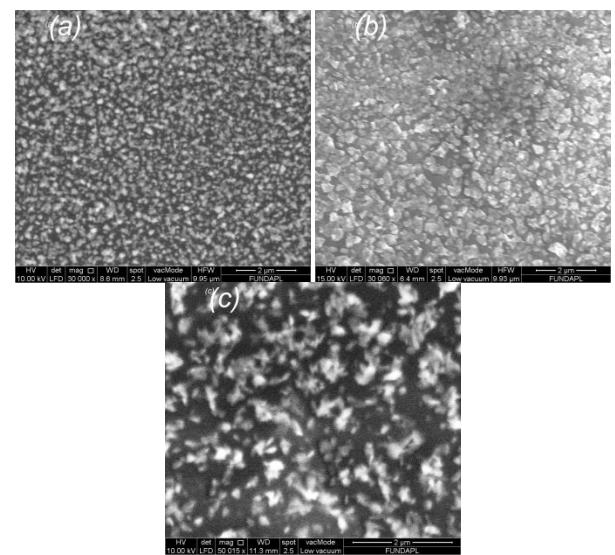
Fig.4. SEM image of CuO thin films at different annealing Temperatures: a)350 °C, b)450°C, c)550°C.
