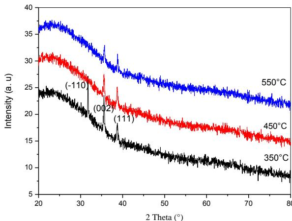
Fig.1. X-ray diffraction patterns of CuO thin films for different annealing temperatures
