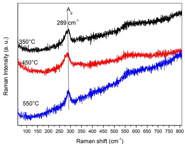
Fig.2. Raman spectra of CuO thin films at different annealing temperatures
