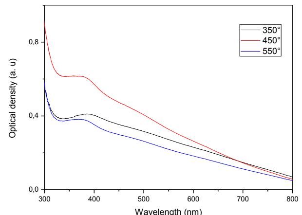
Fig.5. Optical absorption spectra for CuO thin films at different annealing temperatures.
