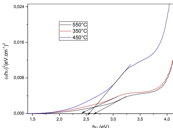
Fig.6. Band gap energy for CuO thin films at different annealing temperatures.
