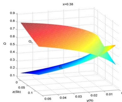
Fig. 3. Rate variation of carrier confinement of electrons and heavy holes concentration as a function of N and Sb for In = 38%.
