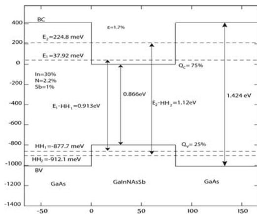
Fig. 5. Band lineup for single quantum well structure GaInAsNSb/GaAs emitting at  $1.3581\mu\text{m}$ .
