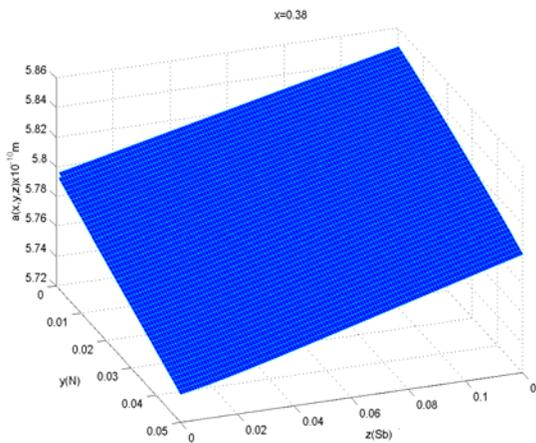
Fig. 1. Lattice parameter variation as a function of the concentration of N and Sb for In = 38%.
