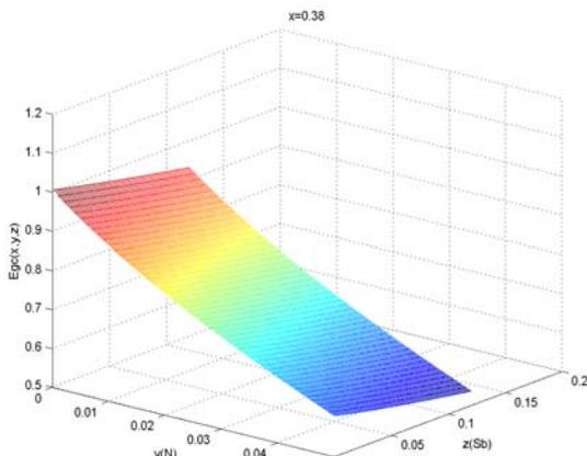
Fig. 4. Variation of the energy of the forbidden band as a function of N and Sb concentrations for In = 38%.
