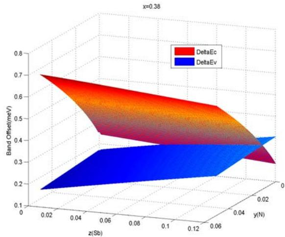
Fig. 2. Shift variation of the energy of conduction and valence bands as a function of N concentration and Sb for In = 38%.
