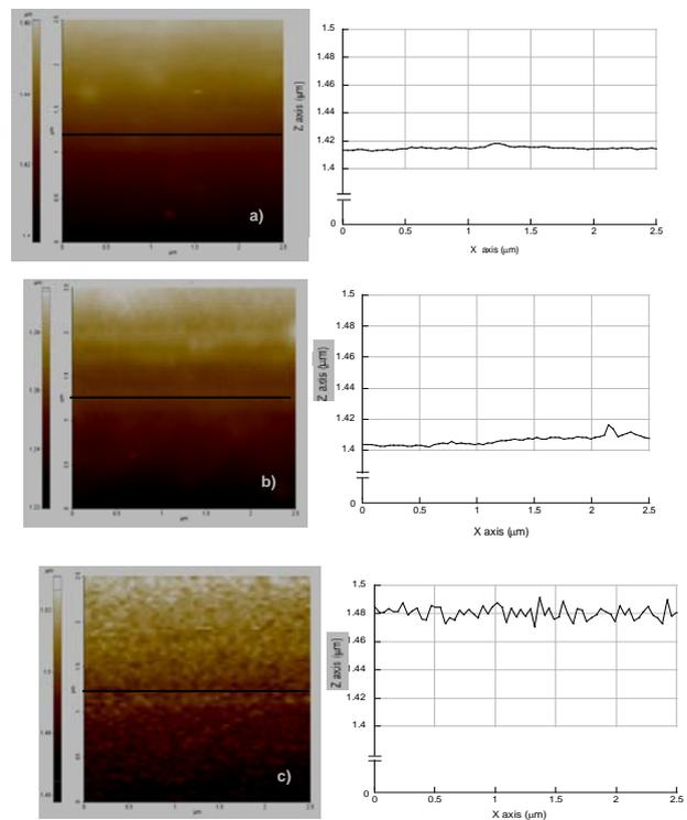
Fig. 3. AFM images showing the surface morphology of blended MEH-PPV:PCBM films at a) 1:1, b) 1:2 and c) 1:4 ratio. The surface profiles (right side) are obtained from line scan along the black line on surface morphology (left side).
