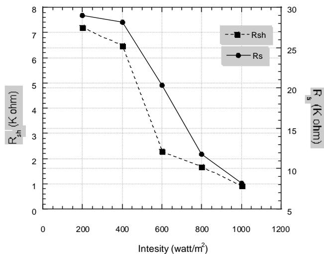
Fig. 6. Effect of the illumination intensity on parallel and series resistances.
