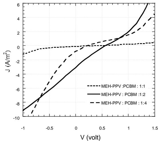
Fig. 2. J-V characteristics for polymer solar cell devices with different ratio of MEH-PPV : PCBM under illumination of  $1000 \text{ W/m}^2$ .
