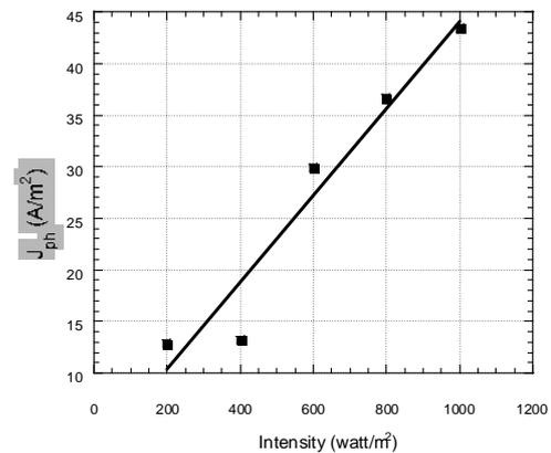
Fig. 5. Curve of photocurrent density and illumination intensity.
