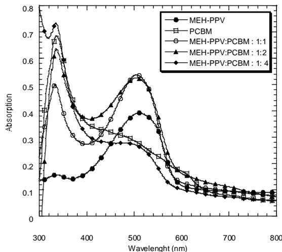
Fig. 1. Absorption spectra for MEH-PPV : PCBM films with different ratio including pure MEH-PPV and pure PCBM spectra.
