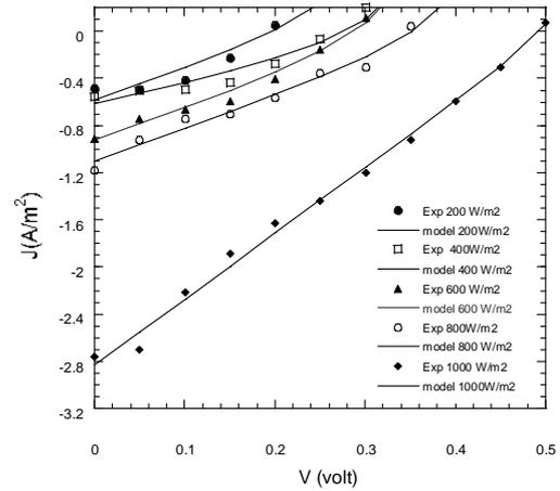
Fig. 4.  $J$ - $V$  characterization curve of experimental and modeling results of solar cells with the structure of glass/ITO/PEDOT:PSS/MEH-PPV:PCBM/Al with variations of light intensity. Ratio of MEH-PPV:PCBM is chosen at 1:2.
