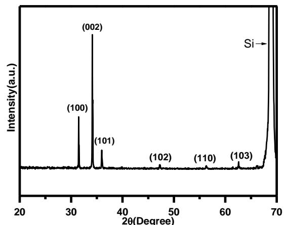
Fig.1. Powder X-ray diffraction pattern of ZnO rods with 0.1M zinc concentration grown at 90°C for 5 h.
