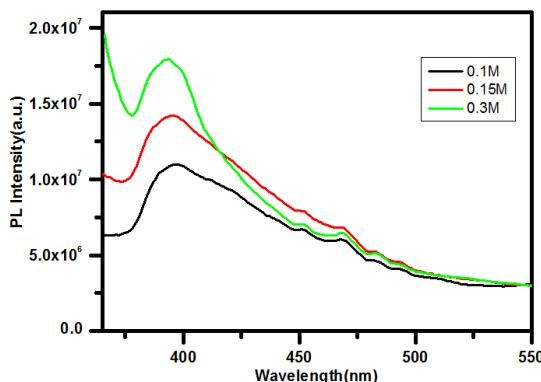
Fig.7 Room temperature PL spectrum of ZnO rod arrays with different precursor concentrations
