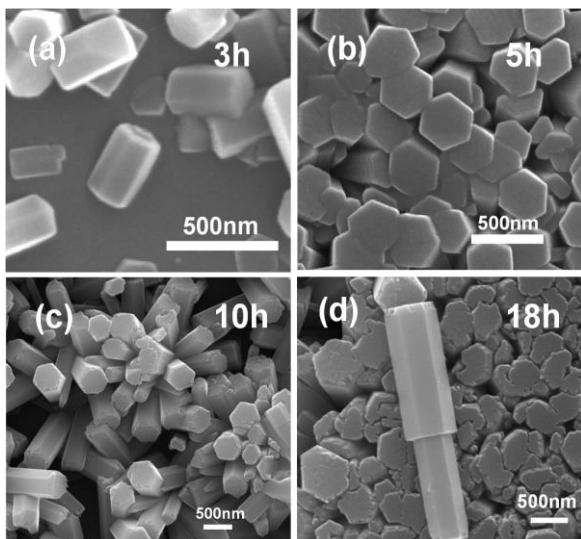
Fig.4 HRSEM images of ZnO rods (0.05M zinc concentration) grown at 90°C for 3 h,5 h,10 h and 18 h
