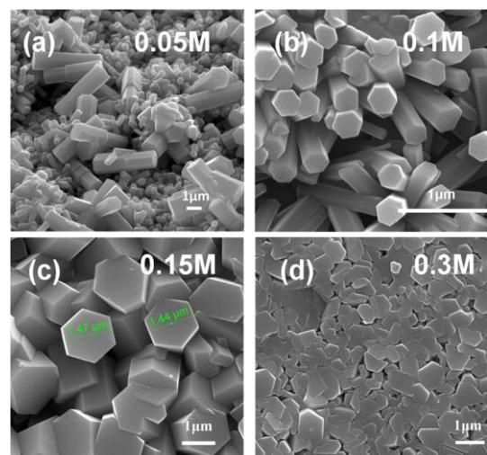
Fig.2 HRSEM images of ZnO rods grown with different precursor concentrations at 90°C for 5 h
