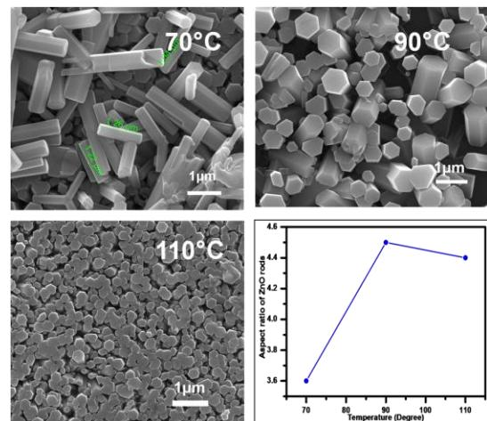
Fig.5 HR-SEM images of ZnO rods grown for different growth temperatures (0.1M zinc concentration) with growth time of 5h and plot of aspect ratio of ZnO rods vs. growth temperature.
