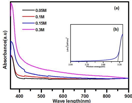
Fig.6 Optical absorbance spectra of ZnO rods with different concentrations. Inset Plot of  $(ahv)^2$  vs  $h\nu$  of ZnO rod film with 0.1M concentration.
