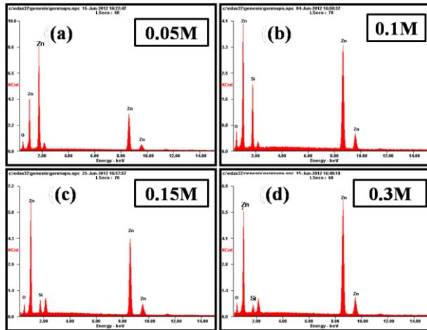
Fig.3 EDAX spectra of ZnO rods with 0.05M ,0.1M ,0.15M, and 0.3M zinc concentrations grown at 90°C for 5 h.
